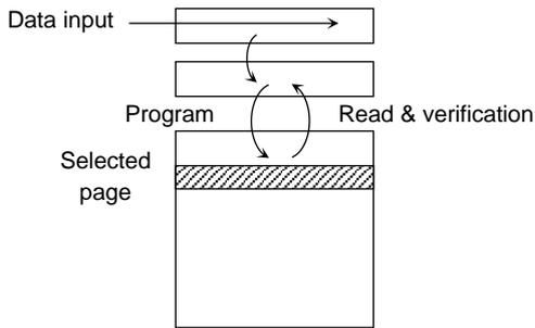
The data is transferred (programmed) from the Data Cache via the Page Buffer to the selected page on the rising edge of WE following input of the "10h" command. After programming, the programmed data is transferred back to the Page Buffer to be automatically verified by the device. If the programming does not succeed, the Program/Verify operation is repeated by the device until success is achieved or until the maximum loop number set in the device is reached.
