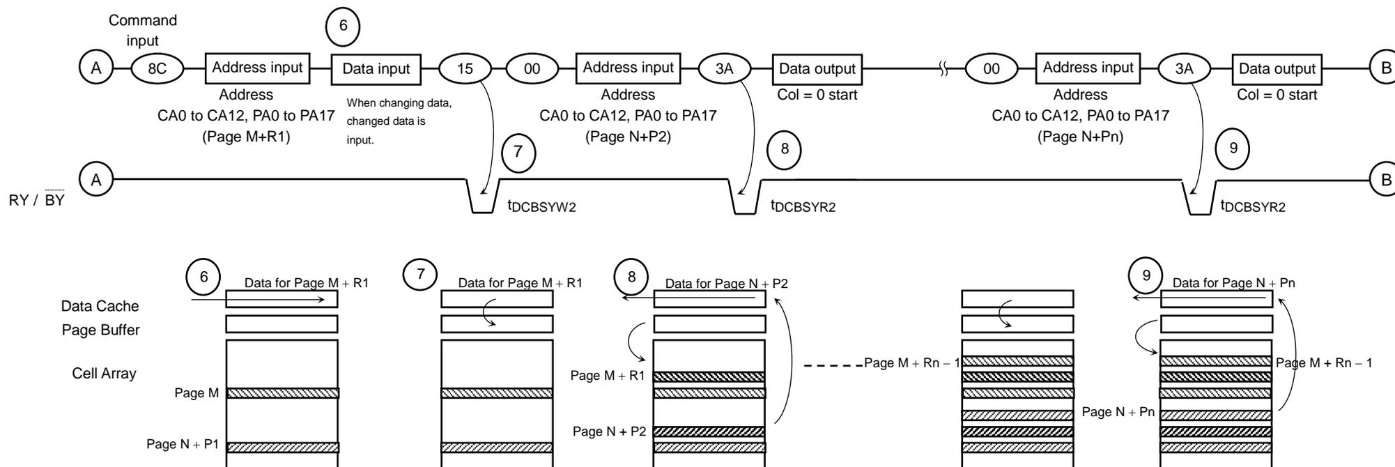
6. Address for Page (M + R1) is input. If the data needs to be changed, changed data is input.
