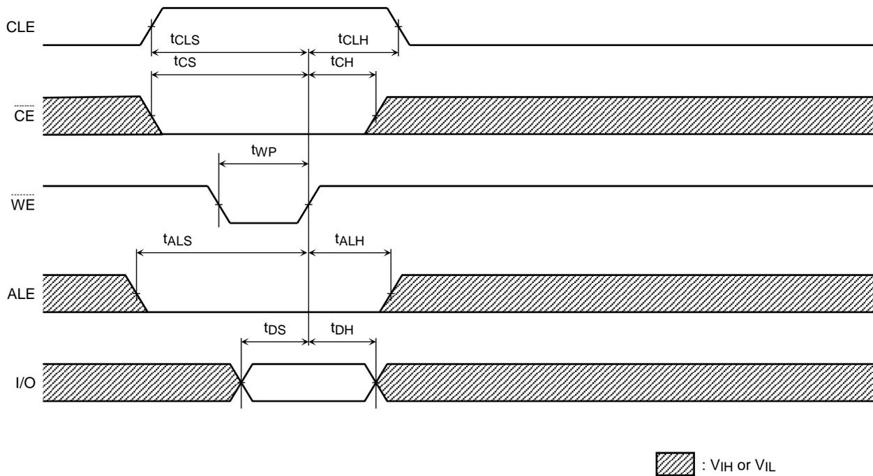
Address Input Cycle Timing Diagram
