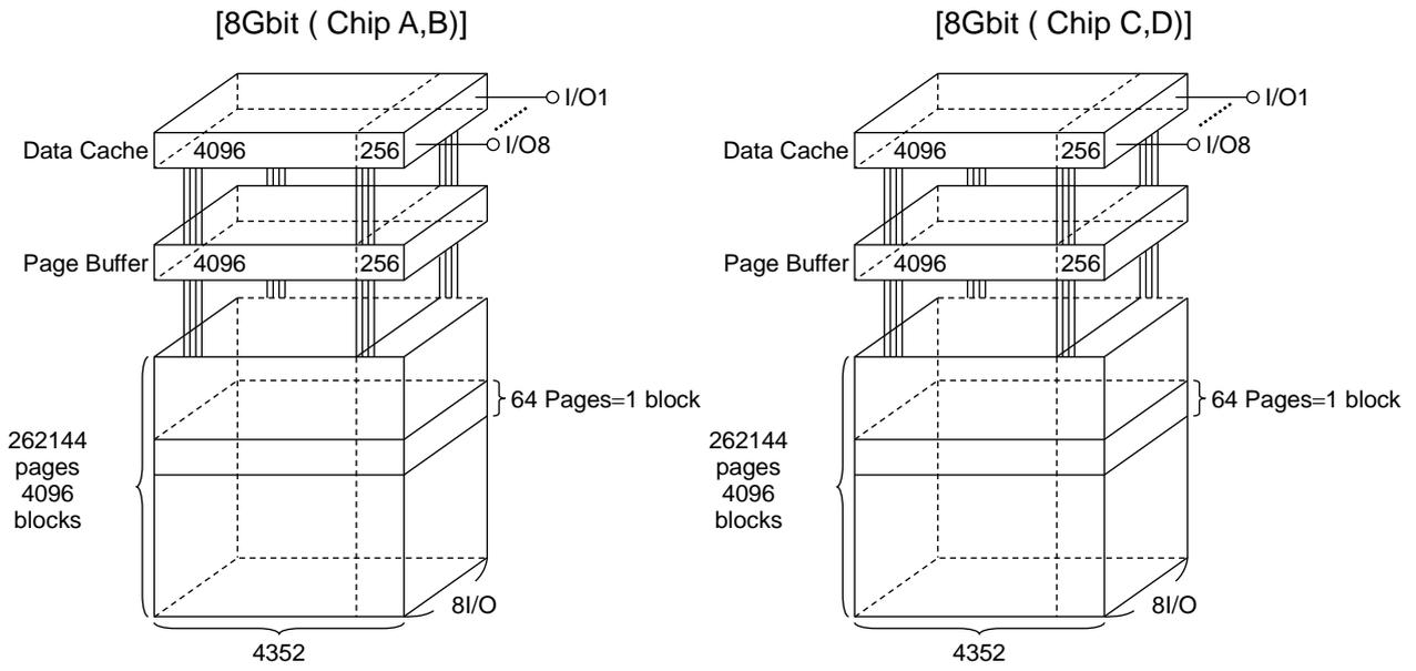
A page consists of 4352 bytes in which 4096 bytes are used for main memory storage and 256 bytes are for redundancy or for other uses.
