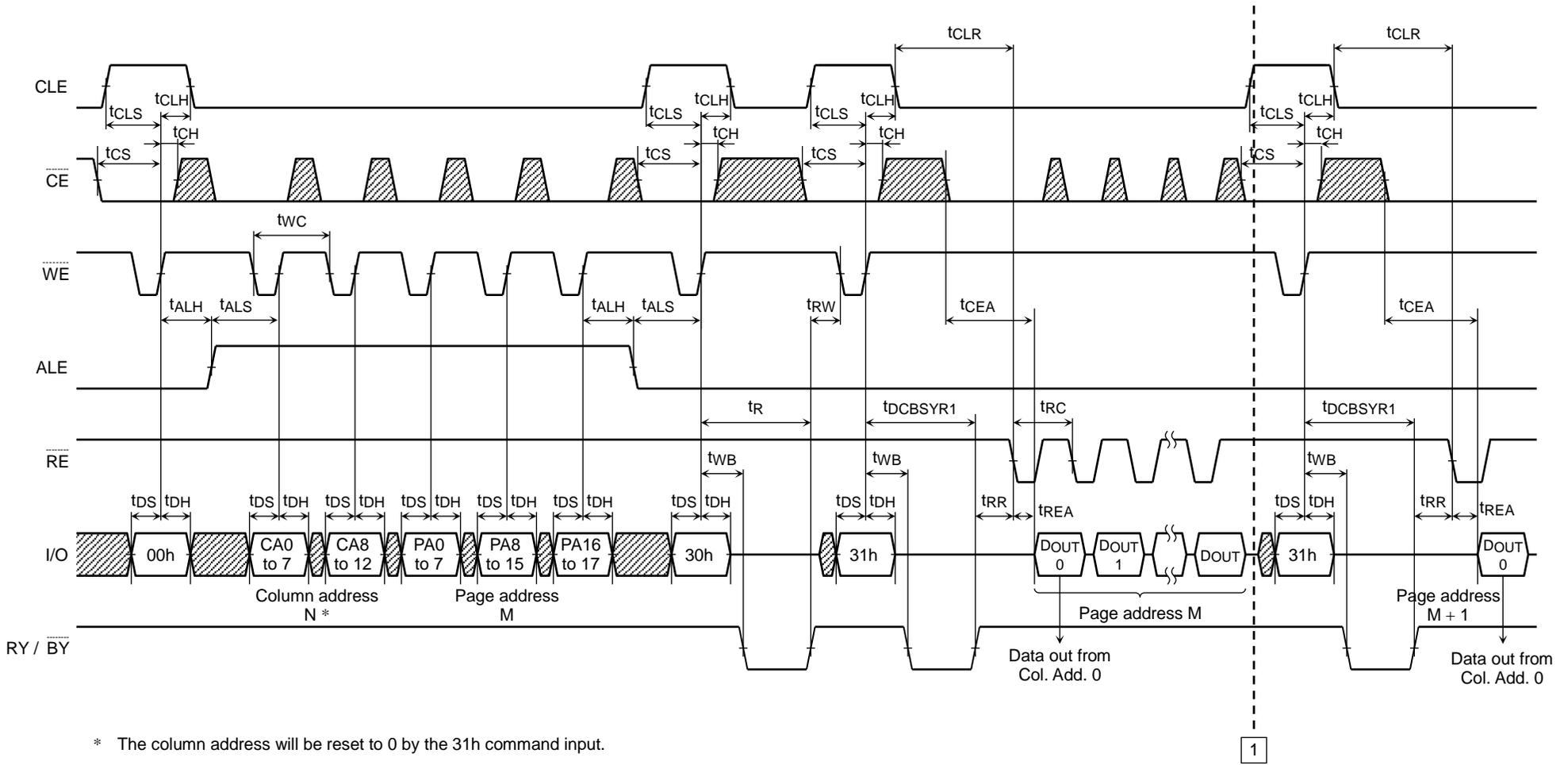
\* The column address will be reset to 0 by the 31h command input.
