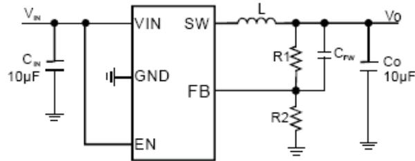
$$V_O = 0.6 \times \left( 1 + \frac{R_1}{R_2} \right)$$
