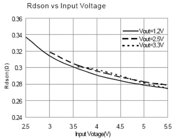
**Typical Performance Characteristics** (cont.) (@ $T_A = +25^\circ\text{C}$ ,  $C_{IN} = 10\mu\text{F}$ ,  $C_O = 10\mu\text{F}$ ,  $L = 4.7\mu\text{H}$ , unless otherwise specified.)
