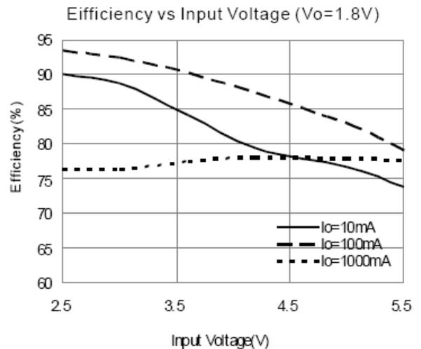
**Typical Performance Characteristics** (cont.) (@ $T_A = +25^\circ\text{C}$ ,  $C_{IN} = 10\mu\text{F}$ ,  $C_O = 10\mu\text{F}$ ,  $L = 4.7\mu\text{H}$ , unless otherwise specified.)
