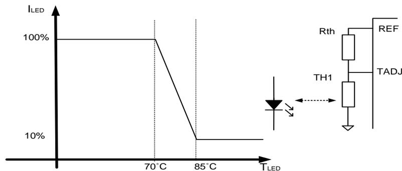
Thermal network response in Buck configuration with:
