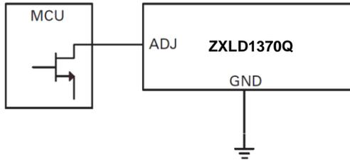
Figure 31 PWM Dimming from MCU
