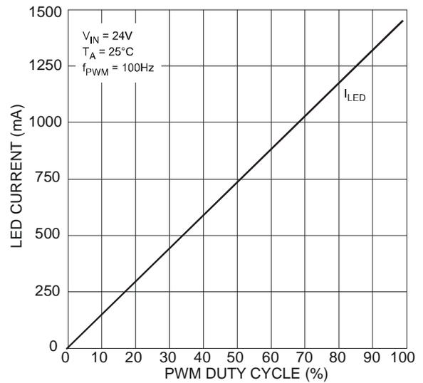
Figure 4 I<sub>LED</sub> vs. PWM Duty Cycle
