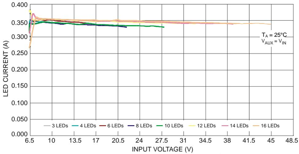
Figure 15  $I_{LED}$  vs. Input Voltage & Number of LED
