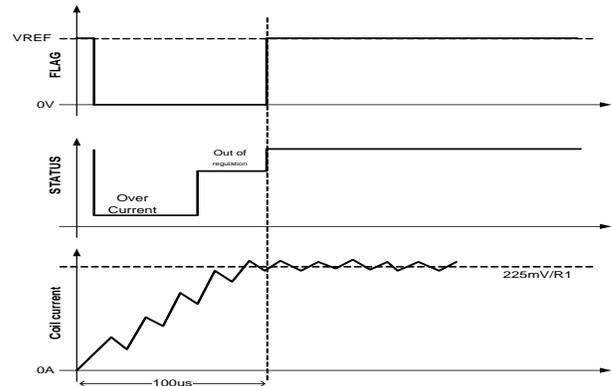
Figure 36 Diagnostic During Start-Up
