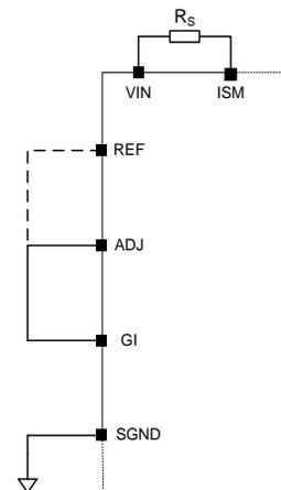
Figure 25 Setting LED Current in Buck Configuration
