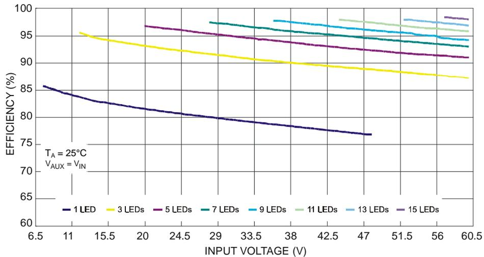
Figure 11 Efficiency vs. Input & Number of LED
