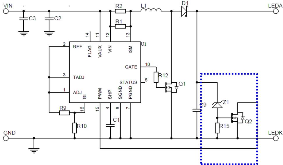
Figure 38 OVP Circuit
