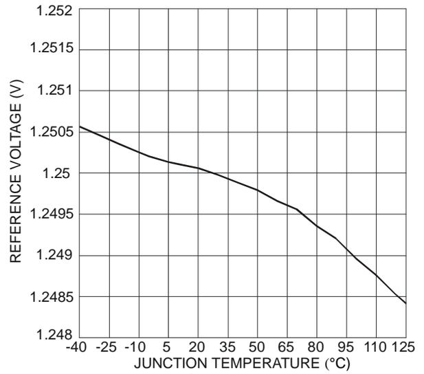
Figure 2 V<sub>REF</sub> vs. Temperature
