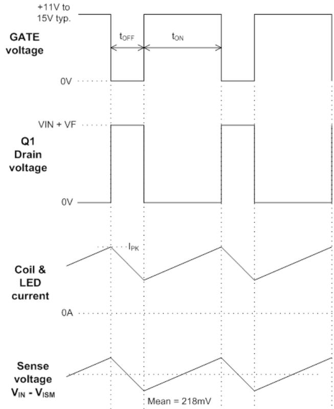
Figure 22 Operating Waveforms (Buck Mode)
