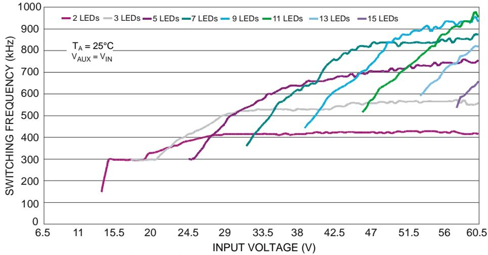
Figure 13 Frequency ZXLD1370Q – Buck Mode –  $L=47\mu H$
