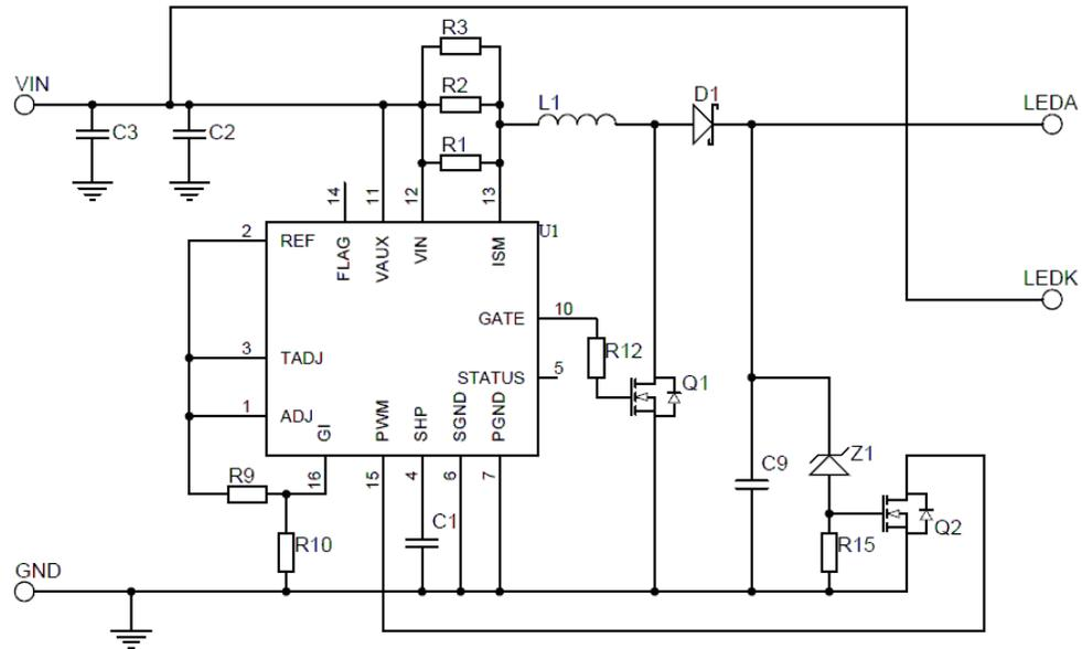
Figure 46 Application Circuit - 700mA Buck-Boost LED Driver
