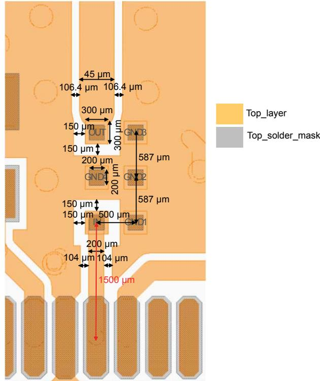
Transmission line between MLPF and antenna is dimensioned to 50 ohms characteristic impedance.
