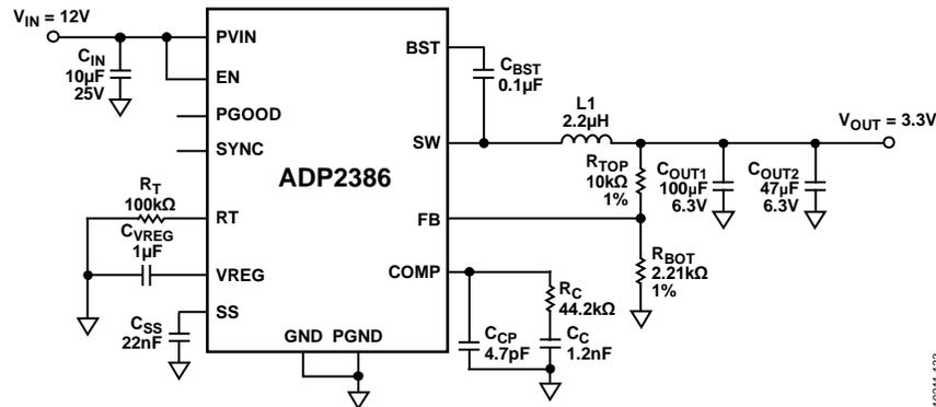
Figure 33. Schematic for Design Example Please change
