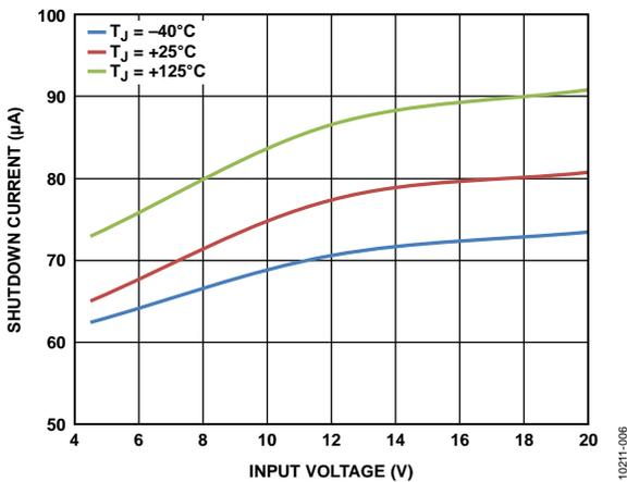
Figure 6. Shutdown Current vs. Input Voltage ( $V_{IN}$ )
