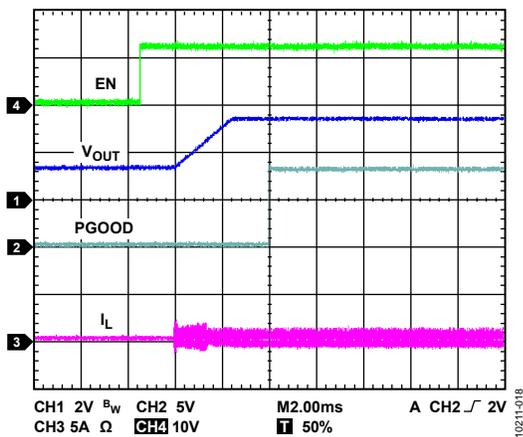
Figure 18. Voltage Precharged Output
