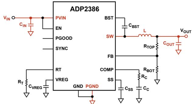
Figure 35. High Current Path in the PCB Circuit
