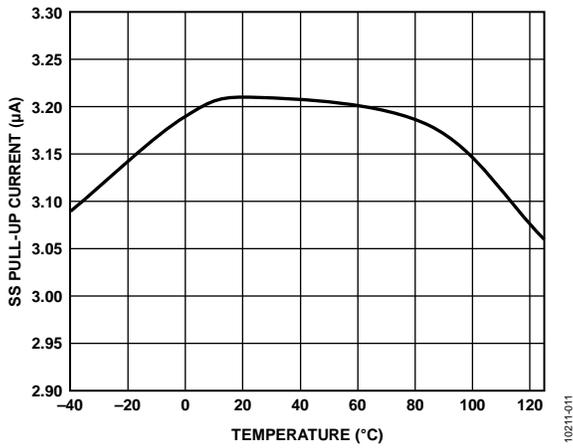
Figure 11. SS Pin Pull-Up Current vs. Temperature
