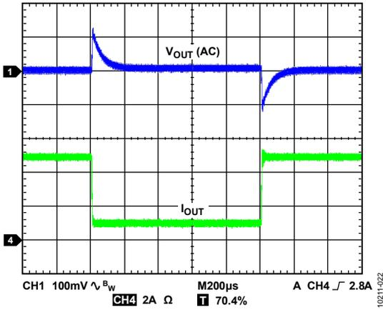
Figure 22. Load Transient Response, 1 A to 5 A
