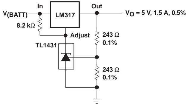
Figure 22. Precision 5-V, 1.5-A, 0.5% Regulator
