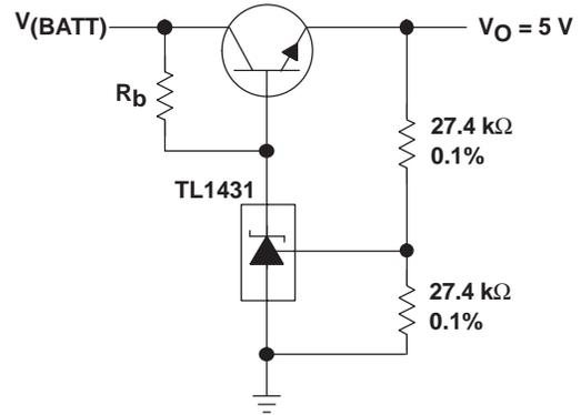
NOTE A:  $R_b$  should provide cathode current  $\geq 1\text{ mA}$  to the TL1431.
