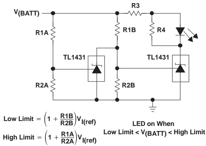
NOTE A: Select R3 and R4 to provide the desired LED intensity and cathode current  $\geq 1$  mA to the TL1431.
