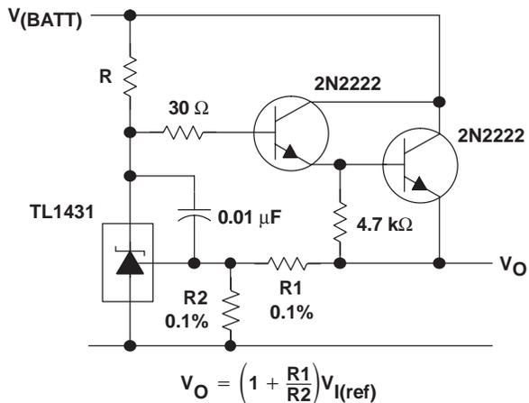
NOTE A: R should provide cathode current  $\geq 1$  mA to the TL1431 at minimum  $V_{(BATT)}$ .
