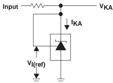
Figure 1. Test Circuit for  $V_{(KA)} = V_{ref}$
