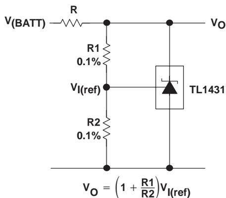
NOTE A: R should provide cathode current  $\geq 1$  mA to the TL1431 at minimum  $V_{(BATT)}$ .
