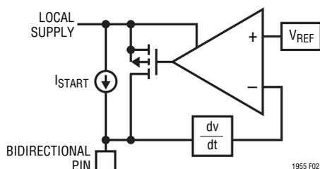
**Figure 2. Dynamic Pull-Up Current Sources**
