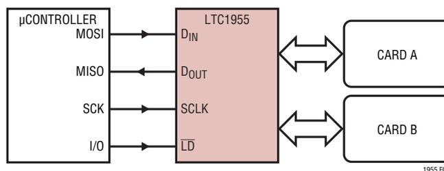
Figure 4. Microcontroller Interface
