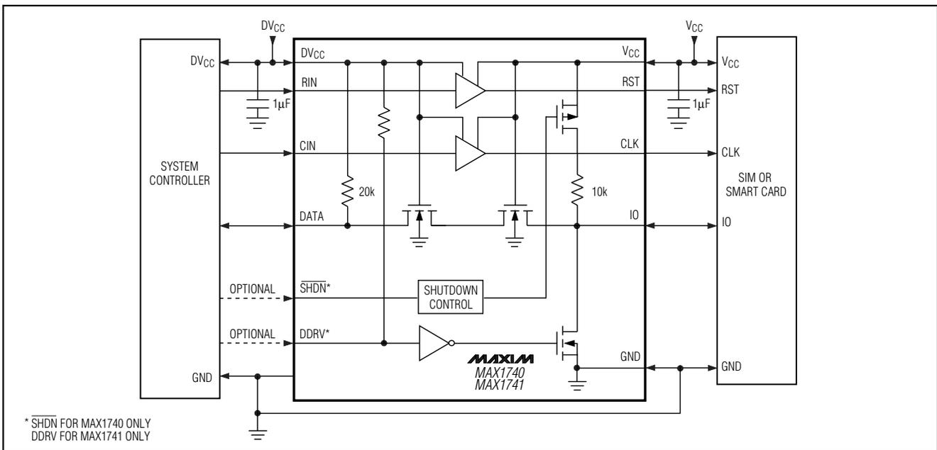
Figure 2. Typical Application Circuit and Functional Diagram
