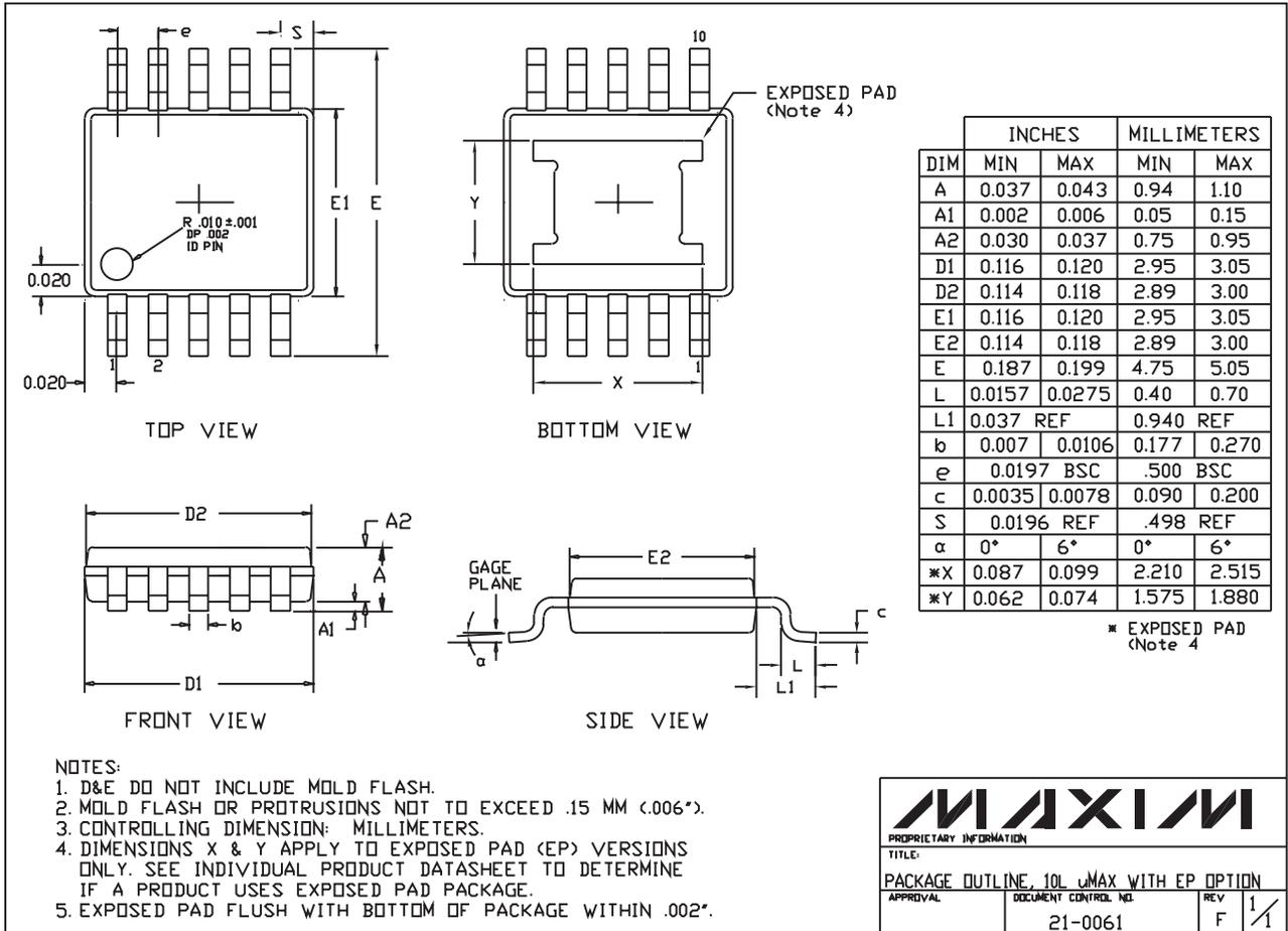
**Note:** The MAX1740/MAX1741 do not have an exposed pad.
