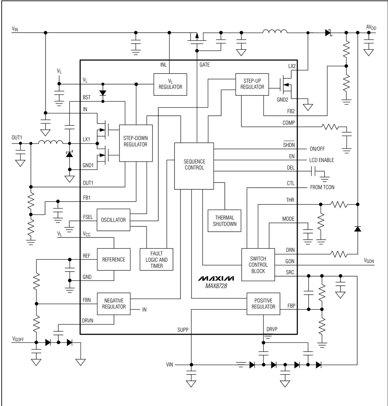
Figure 2. Functional Diagram
