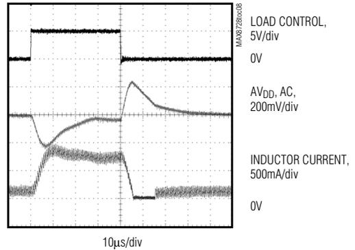
**STEP-UP REGULATOR PULSED-LOAD TRANSIENT RESPONSE (100mA TO 1A)**
