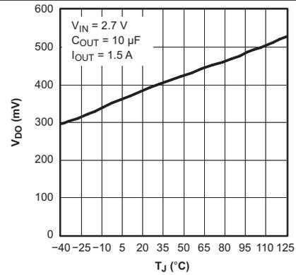
Figure 8. TPS78628 Dropout Voltage vs Junction Temperature
