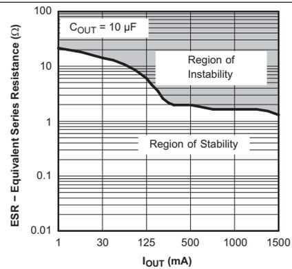
Figure 22. TPS78630 Typical Regions of Stability Equivalent Series Resistance (ESR) vs Output Current
