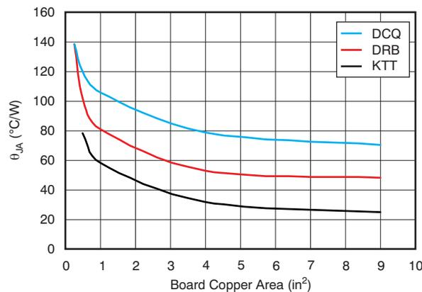
Note:  $\theta_{JA}$  value at board size of 9in<sup>2</sup> (that is, 3in x 3in) is a JEDEC standard.
