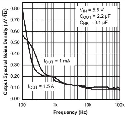
Figure 29. Output Spectral Noise Density vs Frequency
