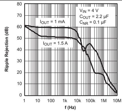
Figure 12. TPS78630 Ripple Rejection vs Frequency
