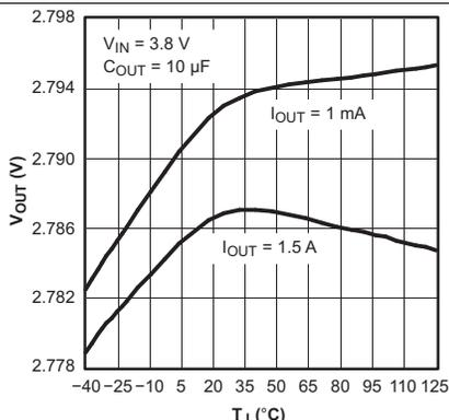
Figure 2. TPS78628 Output Voltage vs Junction Temperature
