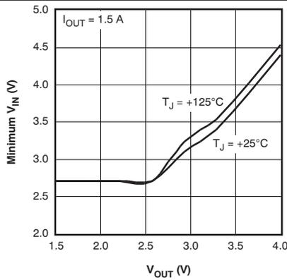
Figure 19. Minimum Required Input Voltage vs Output Voltage
