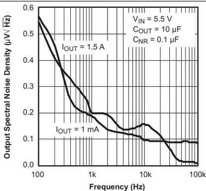
Figure 5. TPS78630 Output Spectral Noise Density vs Frequency
