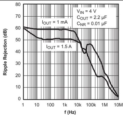
Figure 11. TPS78630 Ripple Rejection vs Frequency
