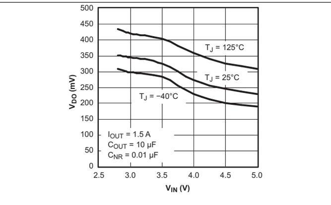
Figure 18. TPS78601 Dropout Voltage vs Input Voltage
