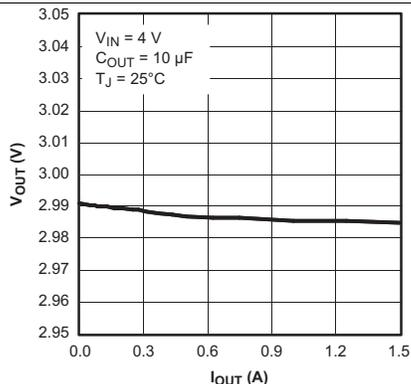
Figure 1. TPS78630 Output Voltage vs Output Current
