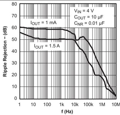
Figure 9. TPS78630 Ripple Rejection vs Frequency
