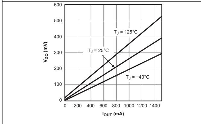
Figure 17. TPS78630 Dropout Voltage vs Output Current
