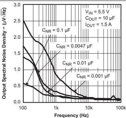
Figure 6. TPS78630 Output Spectral Noise Density vs Frequency
