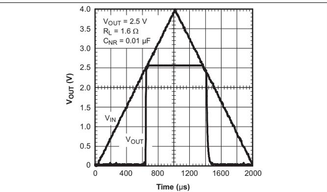
Figure 16. TPS78625 Power Up and Power Down
