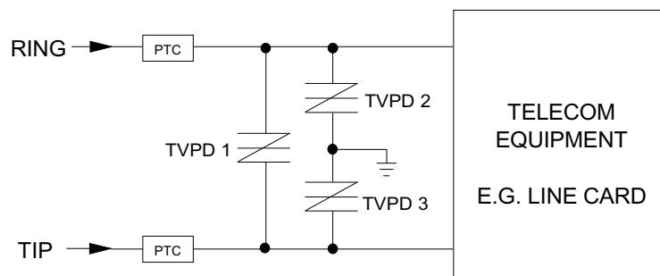
The PTC (Positive Temperature Coefficient) is an overcurrent protection device.
