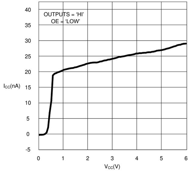
Figure 6-2. SN74HC595 I<sub>CC</sub> vs. V<sub>CC</sub>
