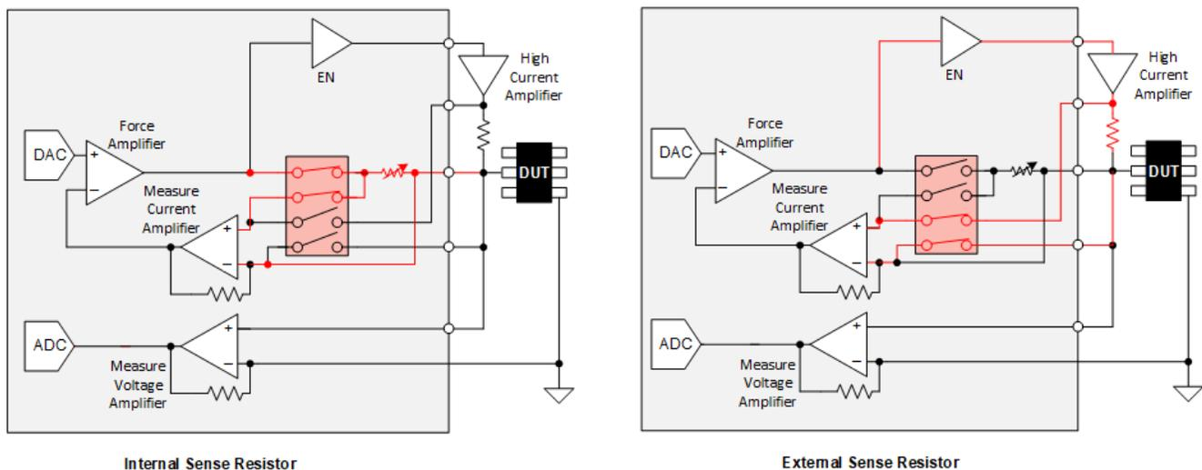
**Figure 10-1. High Current Range Selection Using External Resistor**
