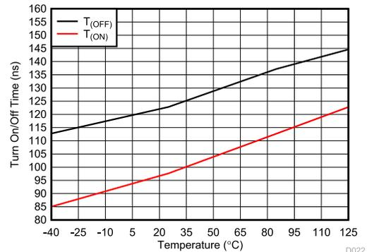
**Figure 7-18.  $T_{ON}$  and  $T_{OFF}$  vs. Temperature**
