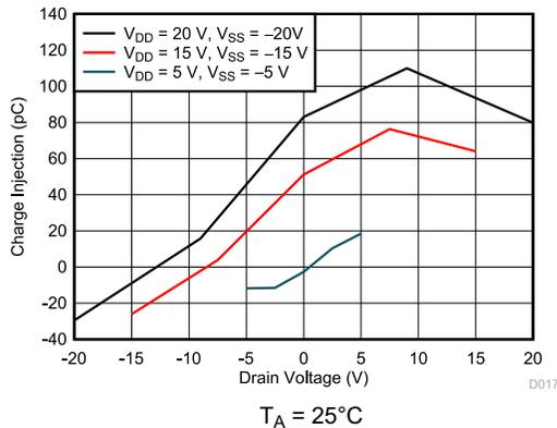
**Figure 10-2. Charge Injection vs. Drain Voltage**
