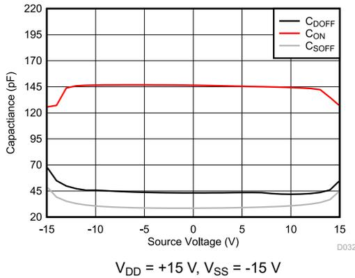
**Figure 7-27. Capacitance vs. Source Voltage or Drain Voltage**
