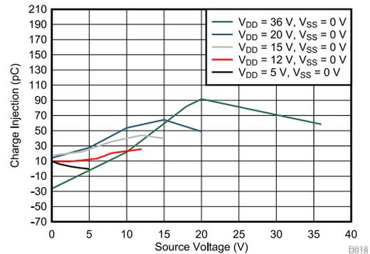
**Figure 7-16. Charge Injection vs. Source Voltage - Single Supply**
