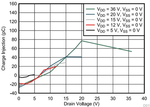
**Figure 7-17. Charge Injection vs. Drain Voltage - Single Supply**
