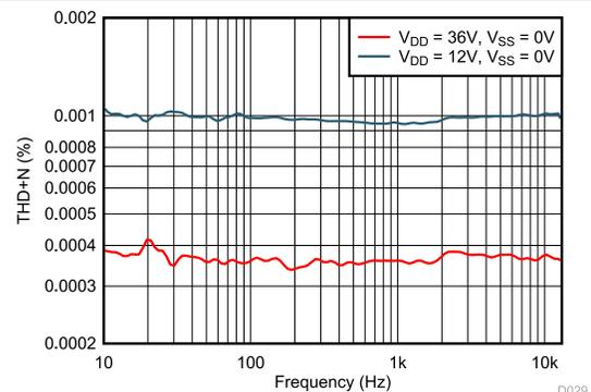
**Figure 7-24. THD+N vs. Frequency (Single Supplies)**
