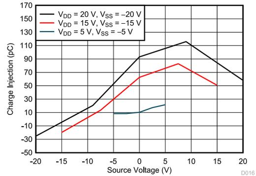
**Figure 7-14. Charge Injection vs. Source Voltage - Dual Supply**
