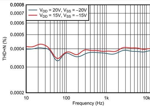
**Figure 7-23. THD+N vs. Frequency (Dual Supplies)**
