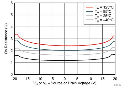
**Figure 7-6. On-Resistance vs Temperature**
