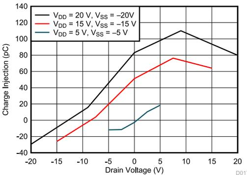
**Figure 7-15. Charge Injection vs. Drain Voltage - Dual Supply**
