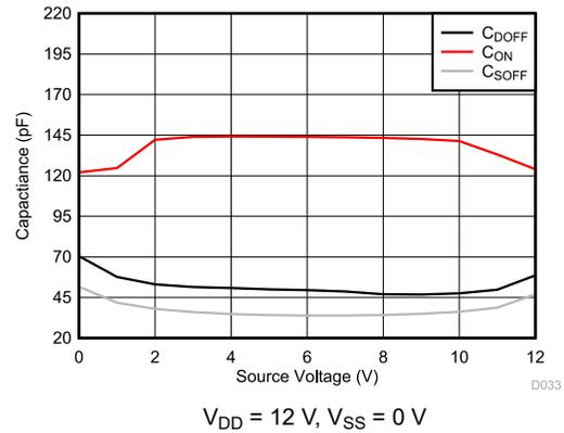
**Figure 7-28. Capacitance vs. Source Voltage or Drain Voltage**
