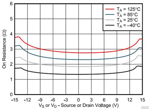
**Figure 7-5. On-Resistance vs Temperature**
