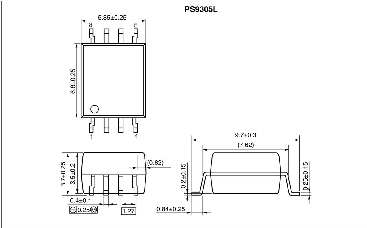
**Lead Bending Type (Gull-wing) for Long Clearance Distance (Surface Mount)**
