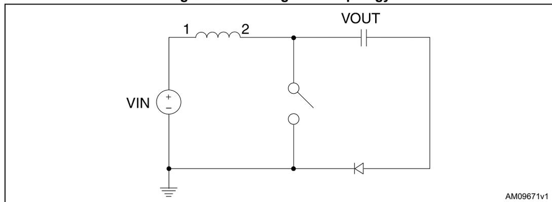
Figure 29. 350 mA LED boost current source
