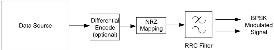
Figure 9 Modulation Process
