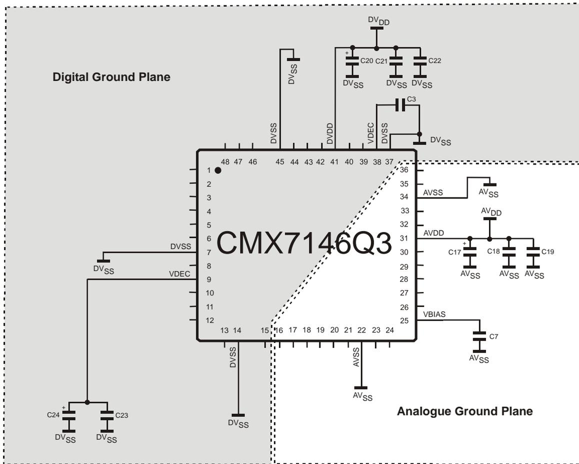
**Figure 3 CMX7146 Power Supply and De-coupling**
