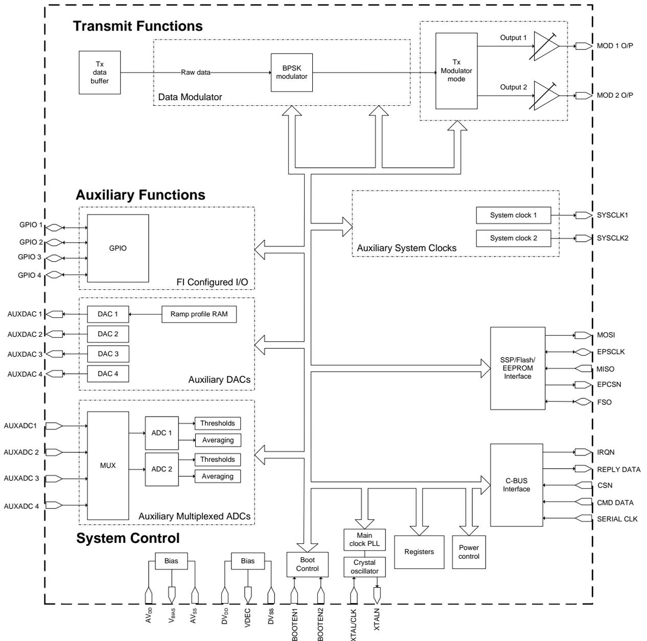
Figure 1 Block Diagram
