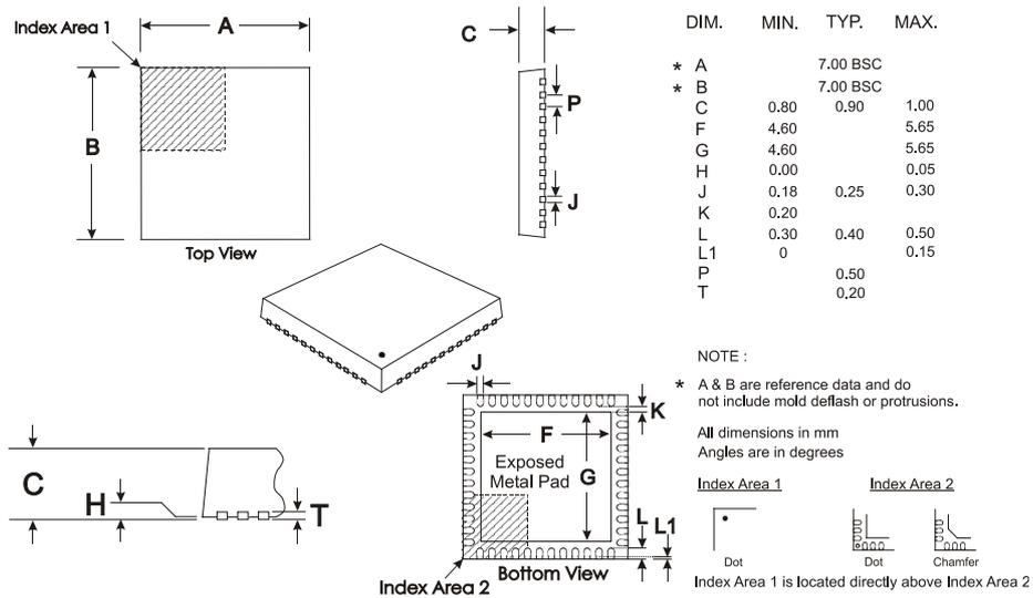
Depending on the method of lead termination at the edge of the package, pull back (L1) may be present. L minus L1 to be equal to, or greater than 0.3mm
