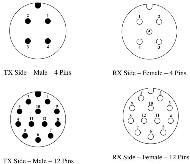
Figure 5.1 – TX and RX mating connector interfaces
