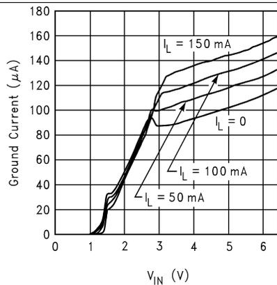
Figure 7. Ground Current vs  $V_{IN}$  at  $-40^\circ C$
