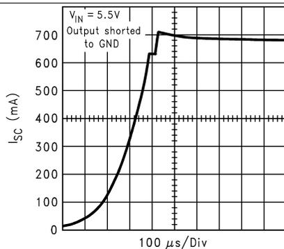
Figure 13. Short Circuit Current (SOT)
