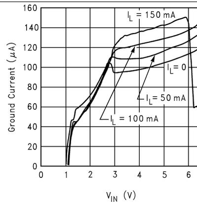
Figure 8. Ground Current vs  $V_{IN}$  at  $125^\circ C$
