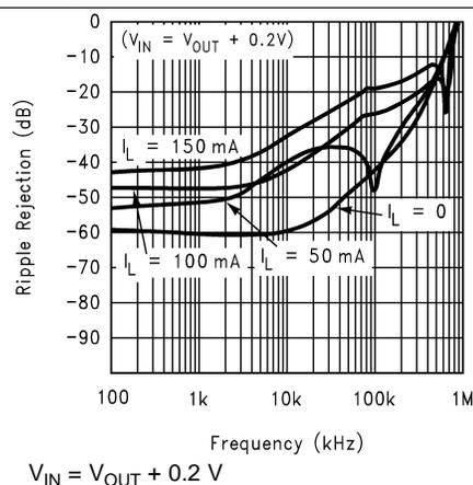
Figure 18. Ripple Rejection
