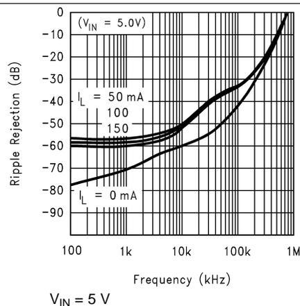
Figure 20. Ripple Rejection
