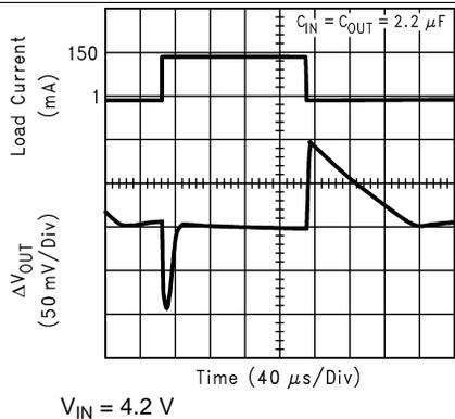
Figure 31. Load Transient Response
