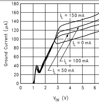
Figure 6. Ground Current vs  $V_{IN}$  at  $25^\circ C$
