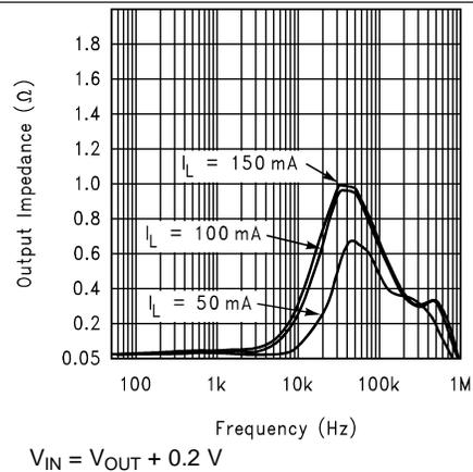
Figure 36. Output Impedance
