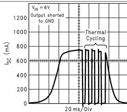
Figure 14. Short Circuit Current (SOT)
