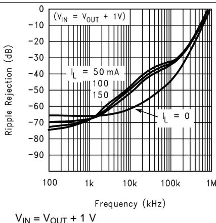
Figure 19. Ripple Rejection
