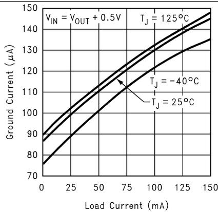
Figure 5. Ground Current vs Load Current
