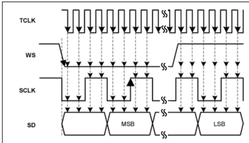
Figure 1. Sampling of I<sup>2</sup>S input signals.
