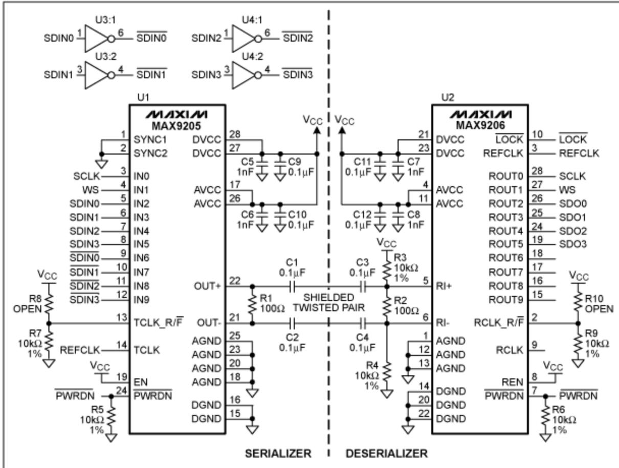
Figure 2. Schematic diagram for using the MAX9205/MAX9206 to transmit I<sup>2</sup>S audio data.
