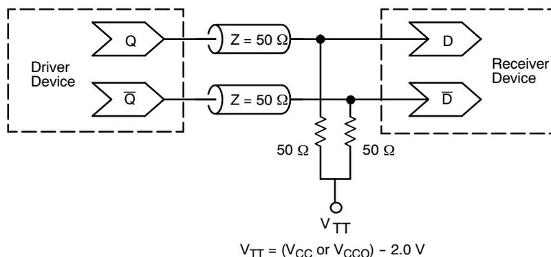
**Figure 4. Typical Termination for Output Driver and Device Evaluation**
