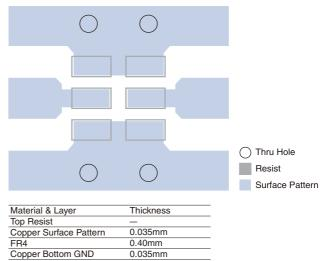
Line width should be designed to match  $50\Omega$  characteristic impedance, depending on PCB material and thickness.
