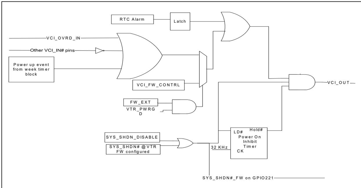
The VCI\_INx# Logic in the block diagram is illustrated in the following figure:
