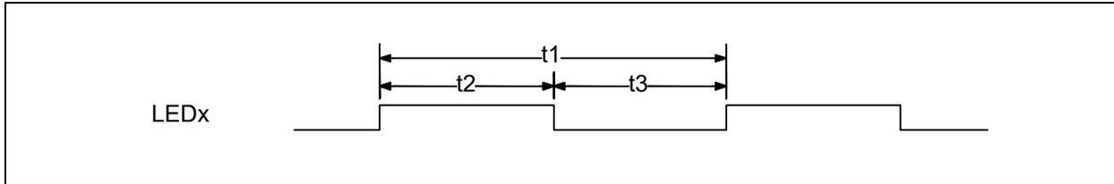
**TABLE 34-8: BLINKING/BREATHING PWM TIMING PARAMETERS, BLINKING MODE**
