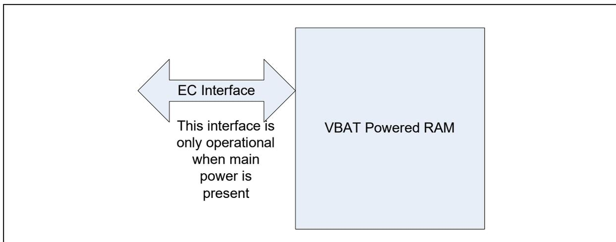
The VBAT Powered RAM provides a 64 Byte Random Accessed Memory that is operational while VTR\_CORE is powered, and will retain its values powered by VBAT while VTR\_CORE is unpowered. The RAM is organized as a 16 words x 32-bit wide for a total of 64 bytes.
