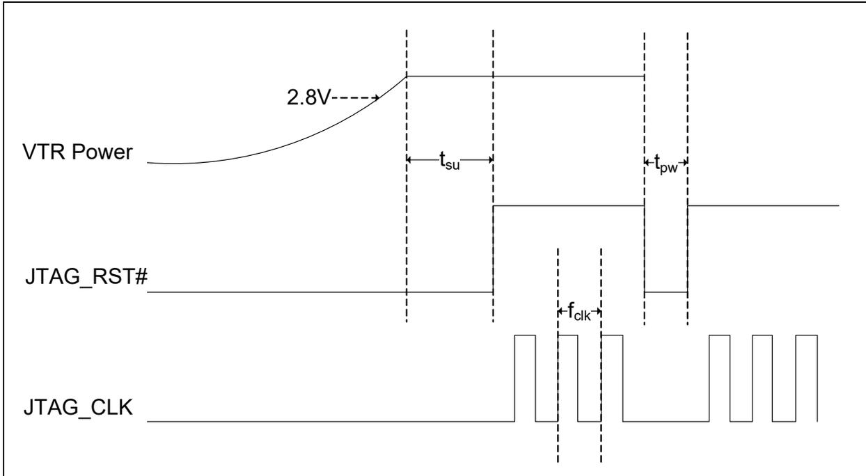
FIGURE 34-13: JTAG SETUP & HOLD PARAMETERS
