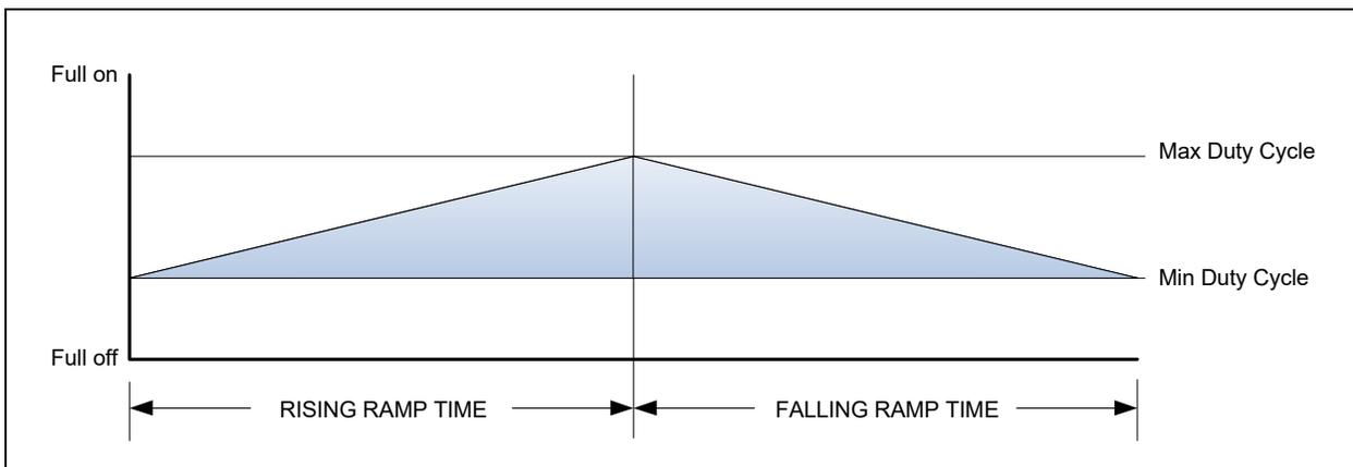
The breathing range of an LED can range between full on and full off, or in a range that falls within the full-on/full-off range, as shown in this figure. The ramp time can be different in different applications. For example, if the ramp time was 1 second, the LED would appear to breathe quickly. A time of 2 seconds would make the LED appear to breathe more leisurely.
