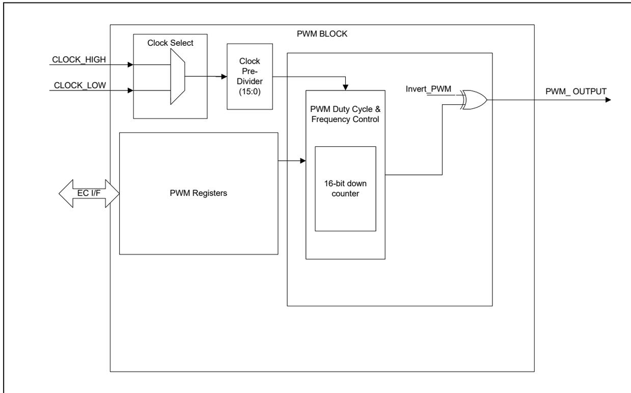
**Note:** In Figure 20-2, the 48MHz clock is represented as CLOCK\_HIGH and the 100KHz clock is represented as CLOCK\_LOW.
