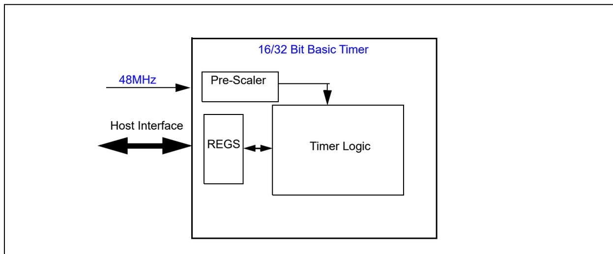
This timer block offers a simple mechanism for firmware to maintain a time base in the design. The timer may be enabled to execute the following features:
