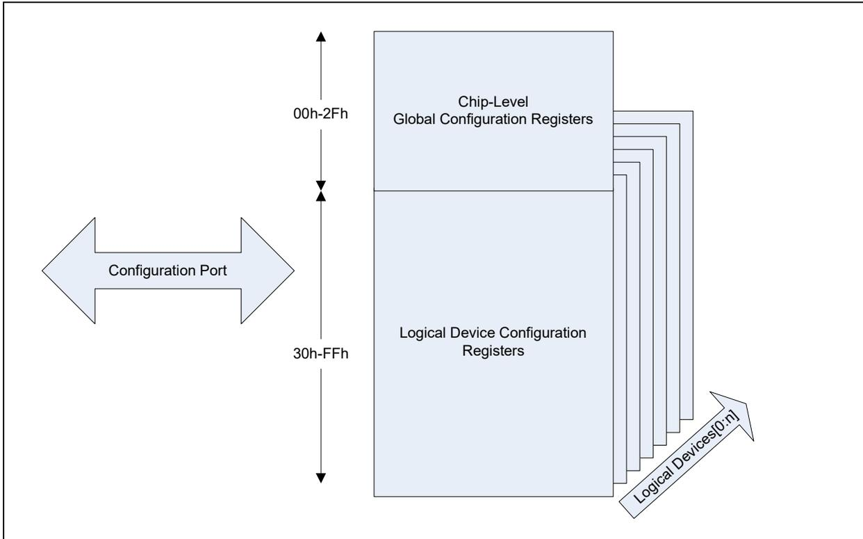
**Note:** Each logical device has a bank of Configuration registers that are accessible at offsets 30h to FFh via the Configuration Port. The Logical Device number programmed in offset 07h determines which bank of configuration registers is currently accessible.
