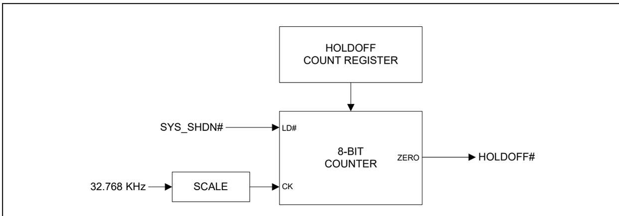
The SCALE function reduces the 32.768KHz clock to 8Hz, so that the 8-bit counter counts intervals of 125ms. The following table shows some of examples of the effect of several settings of the [Holdoff Count Register](#):
