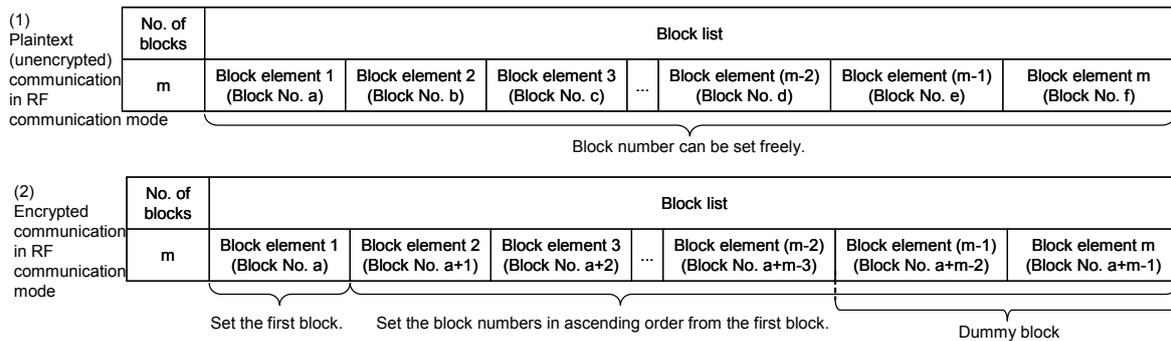
Figure 4-11 Block List Referenced from this RFID
