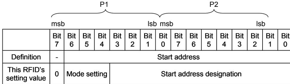
Figure 4-26 Address Specification
