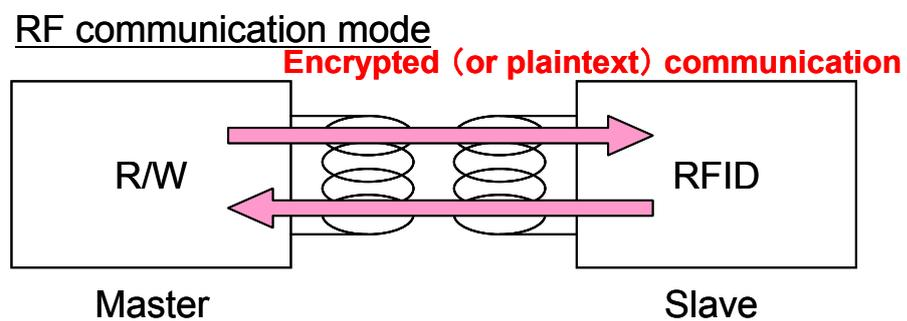
Figure 1-3 Encrypted Communication Function
