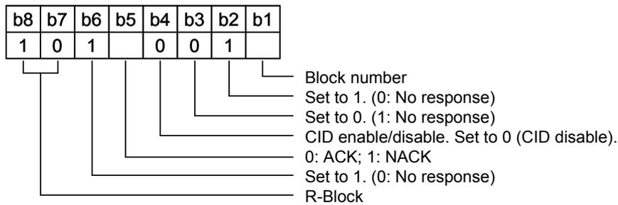
Figure 4-17 R-block Coding
