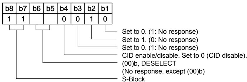
Figure 4-18 S-block Coding
