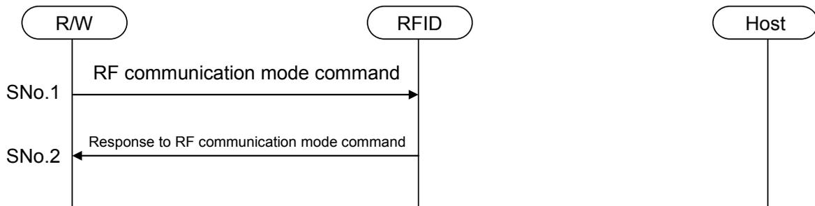
Figure 4-1 RF Communication Mode Sequence
