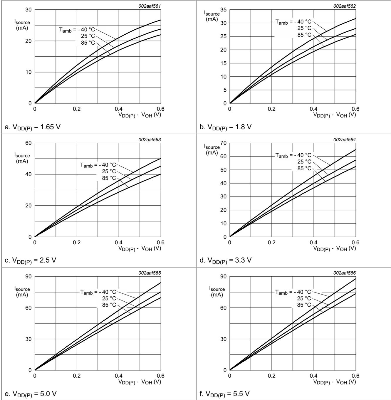
Figure 30. I/O source current versus HIGH-level output voltage with CCX.X = 11b
