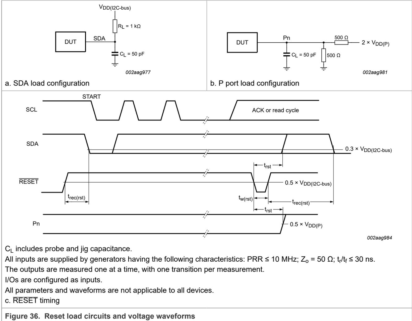
Figure 36. Reset load circuits and voltage waveforms
