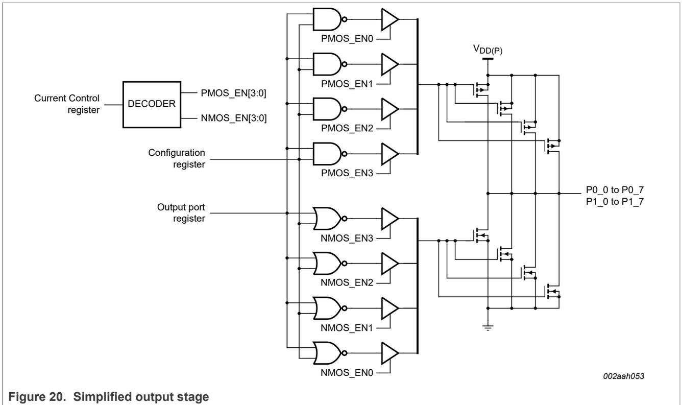
Figure 20. Simplified output stage
