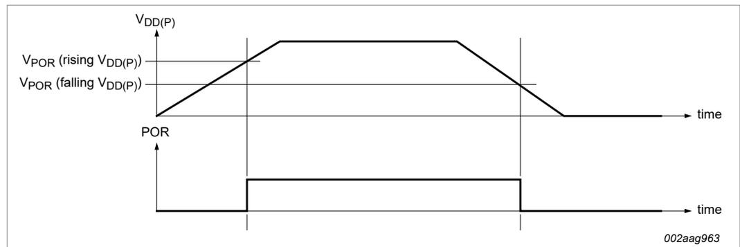
Figure 24. Power-on reset voltage (V<sub>POR</sub>)
