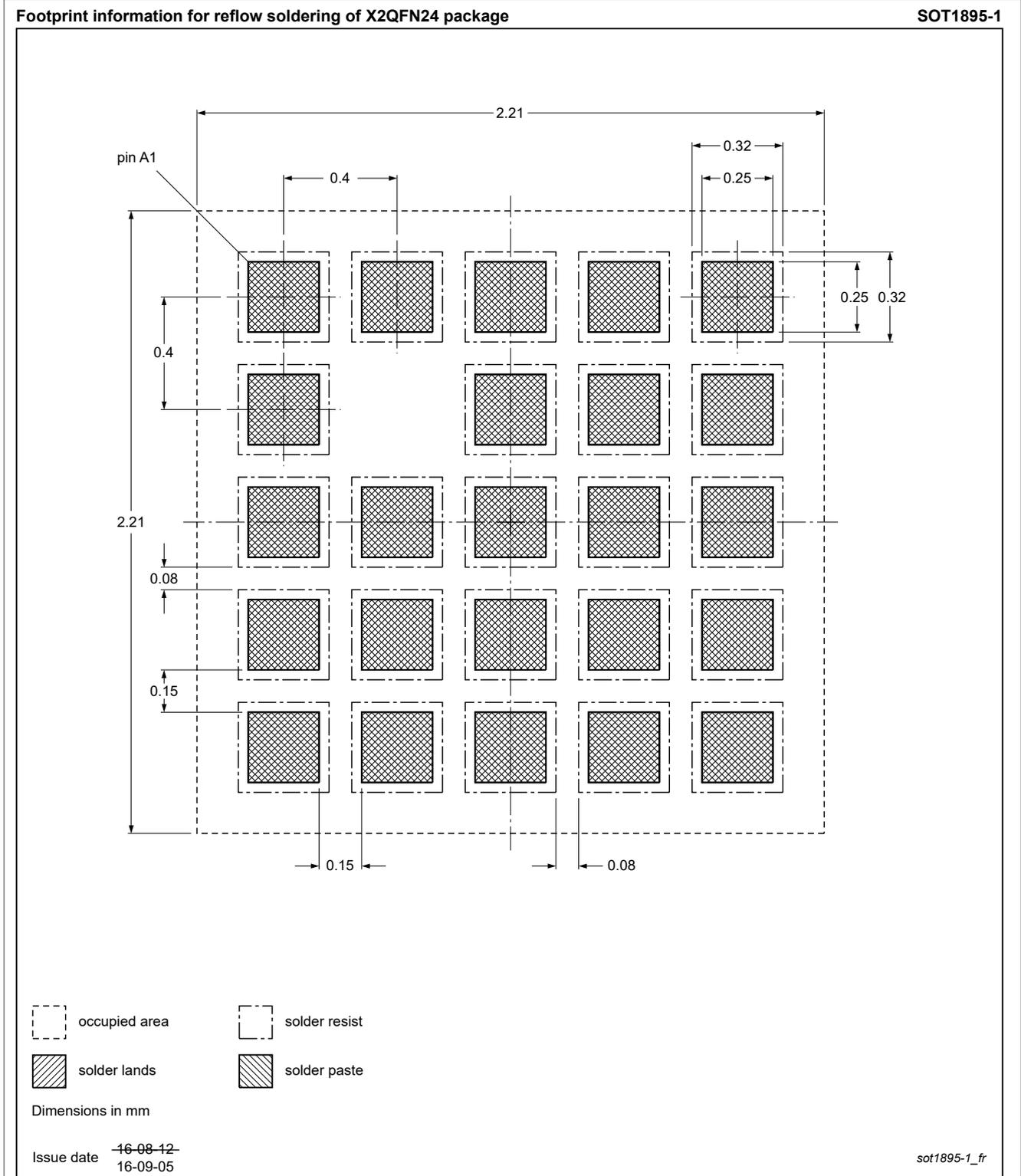
Figure 45. PCB footprint for SOT1895-1 (X2QFN24); reflow soldering
