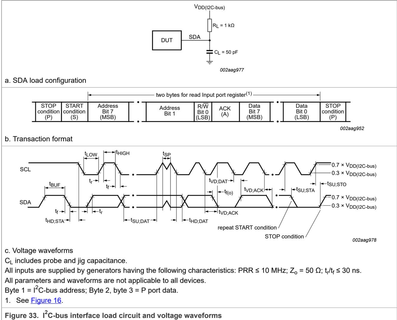
Figure 33. I<sup>2</sup>C-bus interface load circuit and voltage waveforms
