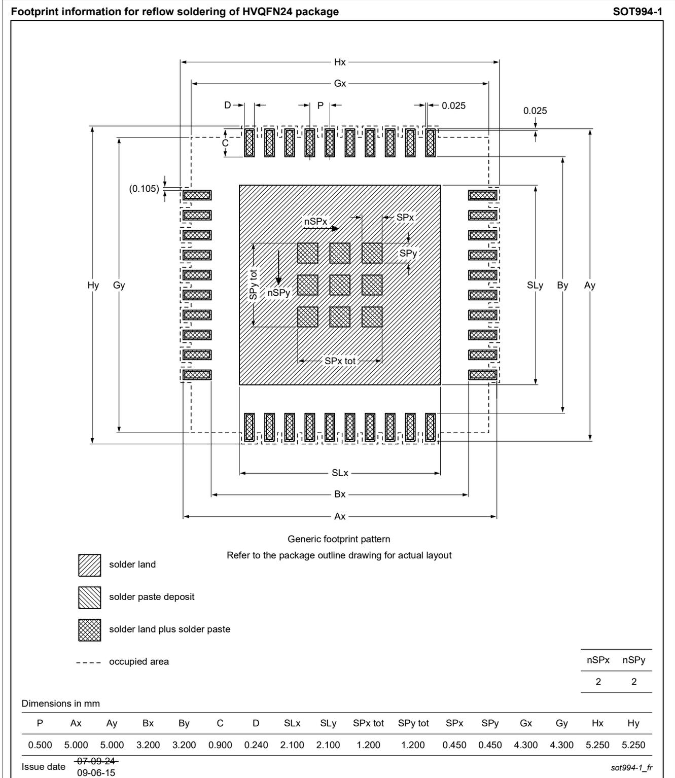
Figure 44. PCB footprint for SOT994-1 (HWQFN24); reflow soldering
