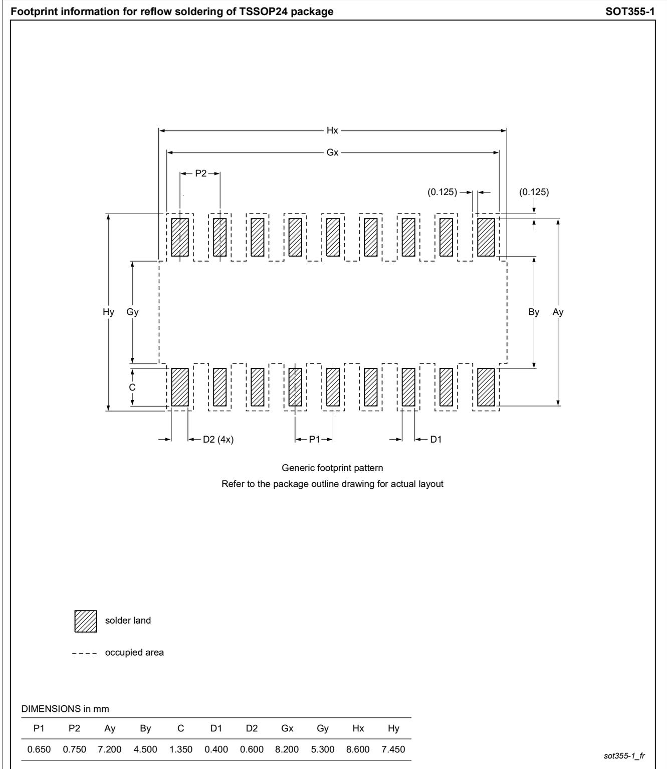
Figure 43. PCB footprint for SOT355-1 (TSSOP24); reflow soldering
