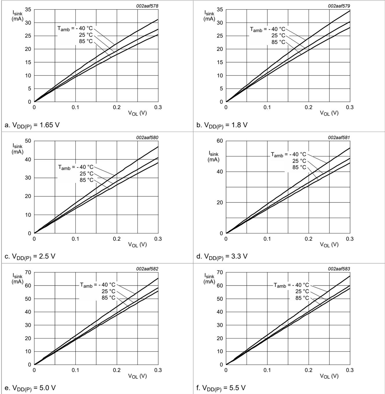
Figure 29. I/O sink current versus LOW-level output voltage with CCX.X = 11b
