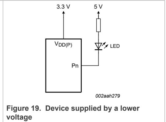
Figure 19. Device supplied by a lower voltage
