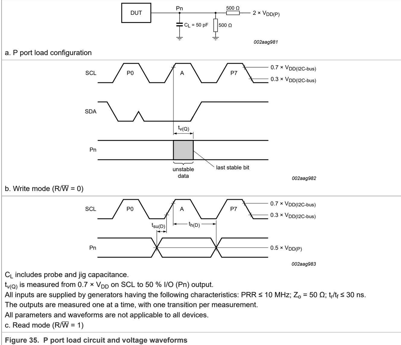
Figure 35. P port load circuit and voltage waveforms
