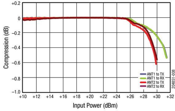
**Figure 8. Compression vs Input Power @ 2.50 GHz and 3 V**
