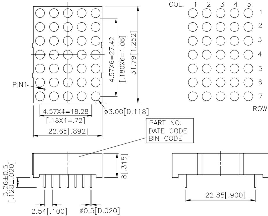
NOTES: All dimensions are in millimeters. Tolerances are ± 0.25 mm (0.01“) unless otherwise noted.
