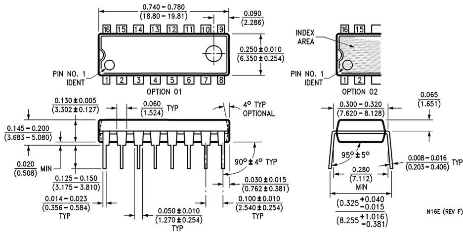
**16-Lead Molded Dual-In-Line Package (N)**
