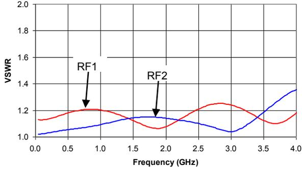
VS<sub>WR</sub> - 15 dB Attenuation vs. Frequency
