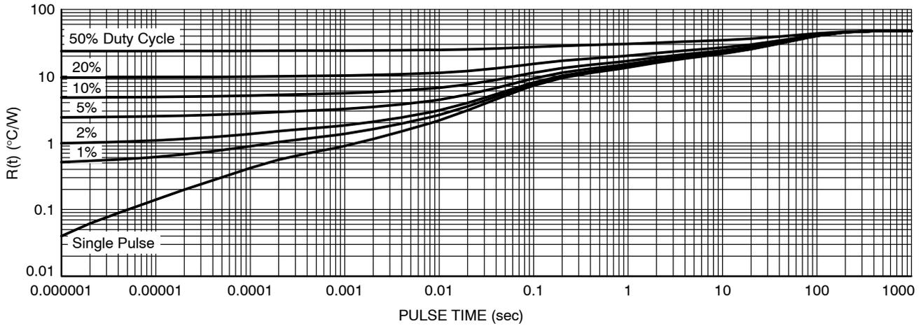
Figure 13. Thermal Characteristics
