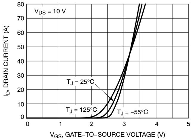
Figure 2. Transfer Characteristics
