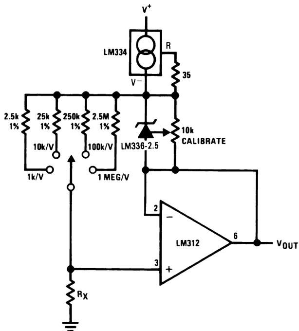
Figure 21. Linear Ohmmeter
