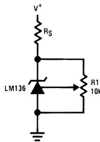
**Figure 14. LM136 With Pot for Adjustment of Breakdown Voltage**
