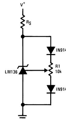
**Figure 15. Temperature Coefficient Adjustment**
