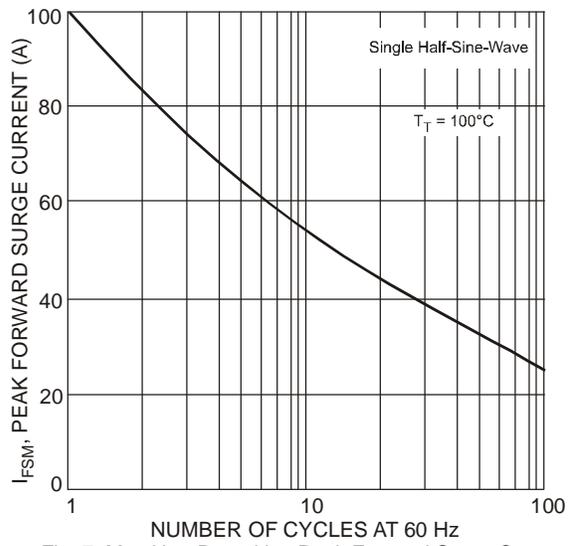
Fig. 7 Max Non-Repetitive Peak Forward Surge Current
