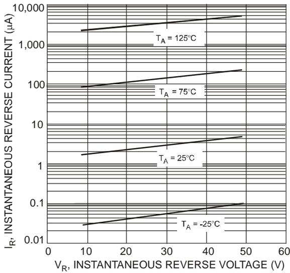
Fig. 3 Typical Reverse Characteristics, B320B-B340B
