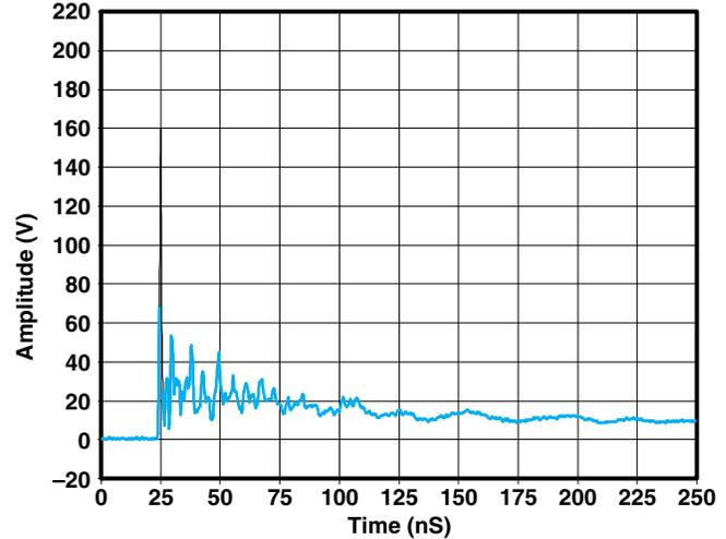
8-kV Contact, Average of Ten Waveforms
