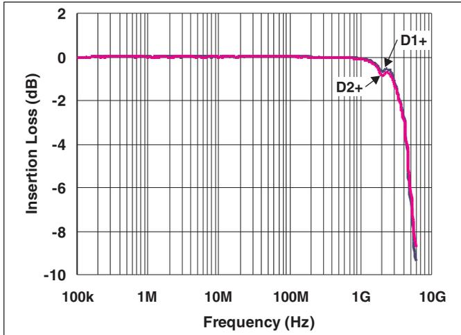
Figure 1. Insertion Loss S21 – I/O to GND
