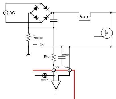
OCL detection is invalid for 170 ns (typ.) after the FET switch turns on (output of PULSE OUT terminal (9 Pin) is high level) to avoid OCL operation introducing errors from needle-like pulse noise generated at the moment the FET switches ON
