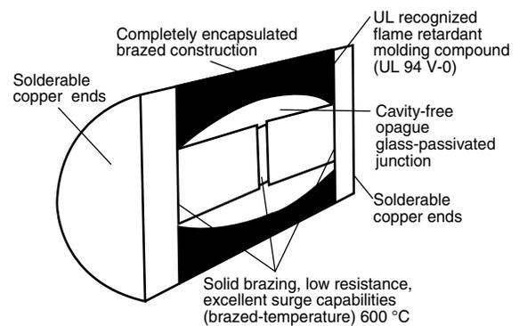
Fig. 1 - SUPERECTIFIER Construction
