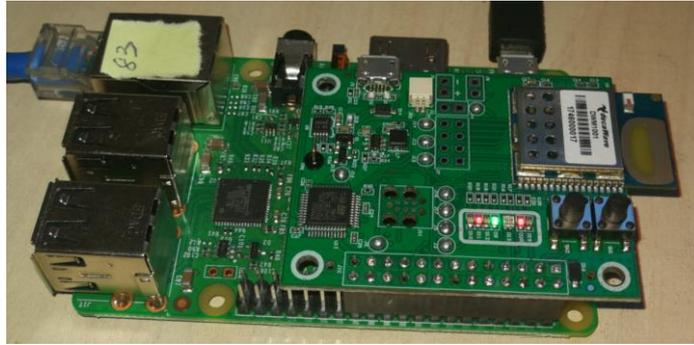
**Figure 9 Connecting DWM1001 to Raspberry Pi 3 over header pins**
