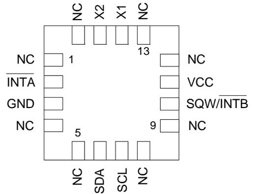
**Pin Assignment (16-pin SOIC)**
