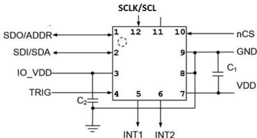
**Figure 1: KX134 Application Schematic**
