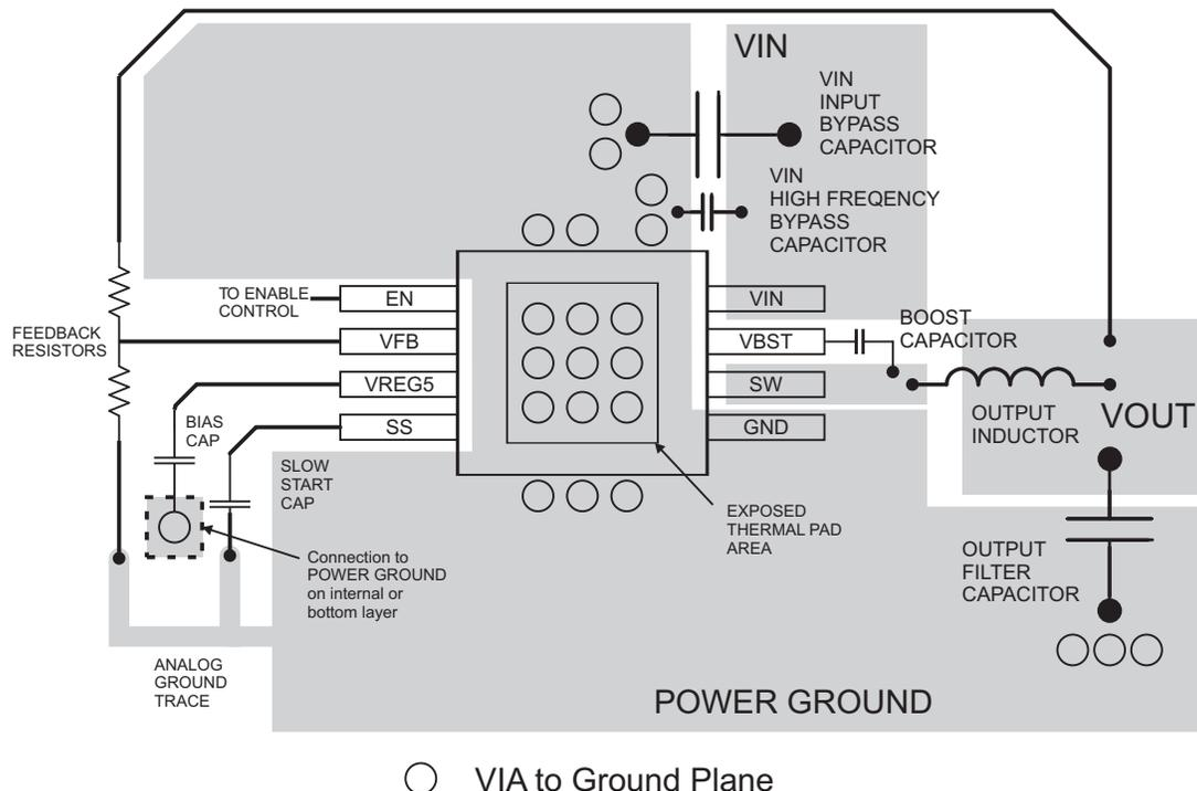
Figure 18. PCB Layout
