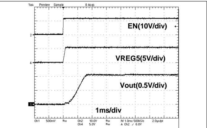
Figure 14. Start-Up Waveform
