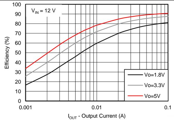
Figure 8. Light Load Efficiency vs Output Current
