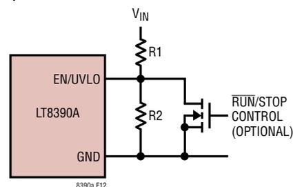
Figure 12. V<sub>IN</sub> Undervoltage Lockout (UVLO)
