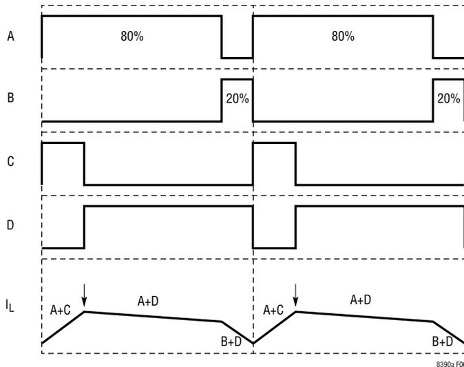
Figure 6. Peak-Boost in Buck-Boost Region ( $V_{IN} \sim V_{OUT}$ )
