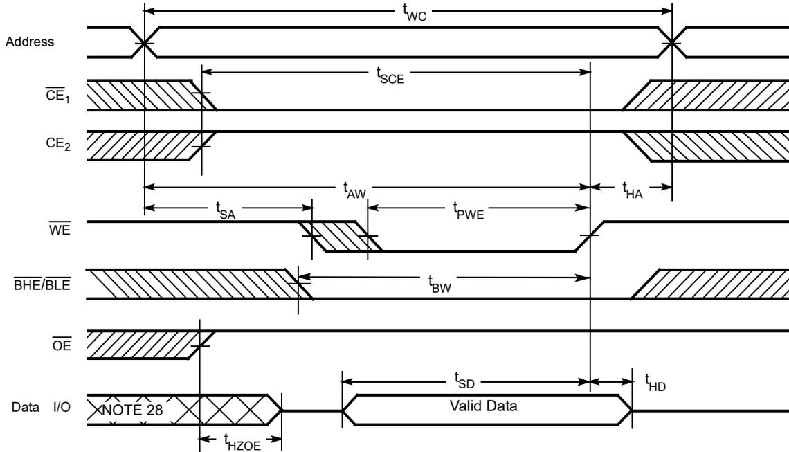
Figure 7. Write Cycle No. 2 ( $\overline{CE}_1$  or  $CE_2$  Controlled) [25, 26, 27]
