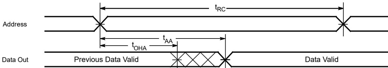
Figure 5. Read Cycle No. 2 ( $\overline{OE}$  Controlled) [23, 24]
