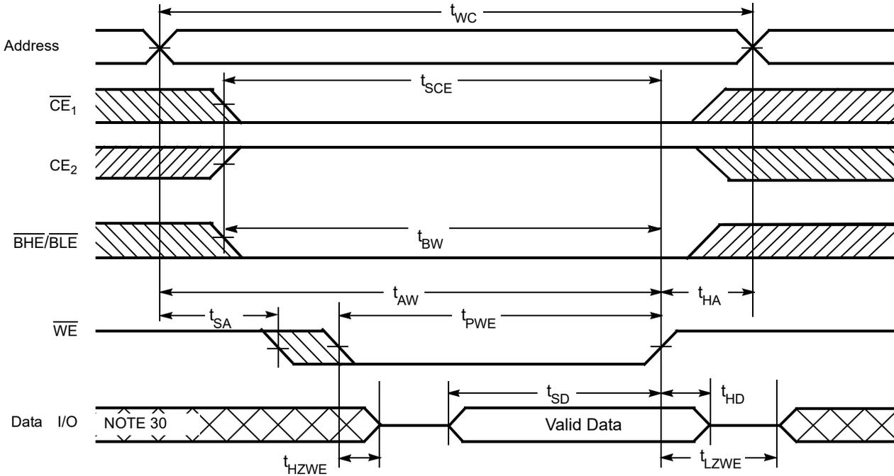
Figure 9. Write Cycle No. 4 ( $\overline{BHE}/\overline{BLE}$  Controlled,  $\overline{OE}$  LOW)<sup>[29]</sup>
