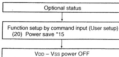
Set the time ( $t_L$ ) from power save to turning off the VDD - VSS power (VDD - VSS = 1.8 V) longer than the time ( $t_H$ ) when the potential of V5 ~ V1 becomes below the threshold voltage (approximately 1V) of the LCD panel.
