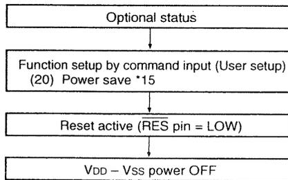
Set the time ( $t_L$ ) from reset active to turning off the VDD - VSS power (VDD - VSS = 1.8 V) longer than the time ( $t_H$ ) when the potential of V5 ~ V1 becomes below the threshold voltage (approximately 1 V) of the LCD panel. For  $t_H$ , refer to the <Reference Data> of this event. When  $t_H$  is too long, insert a resistor between V5 and VDD to reduce it.
