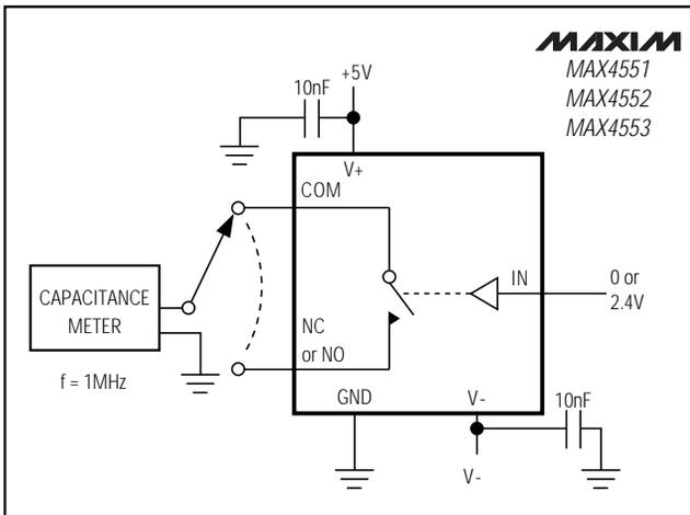
Figure 6. Channel Off-Capacitance
