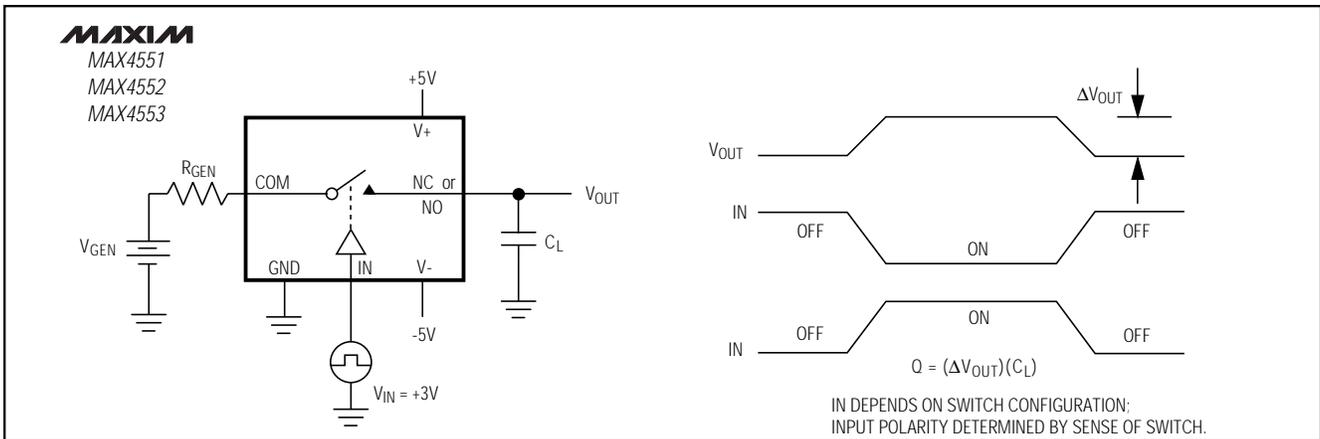
Figure 3. Charge Injection
