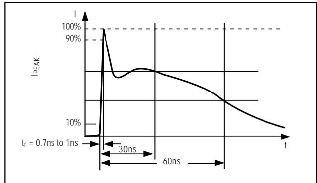
Figure 11. IEC 1000-4-2 ESD Generator Current Waveform
