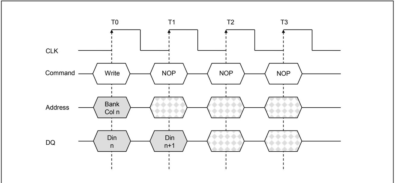
**Figure 15. Write Burst - Burst length of 2**
