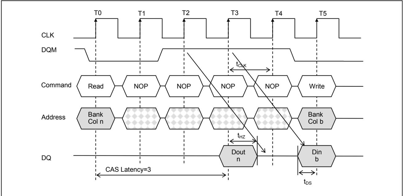
Figure 7. Read to Write with extra clock cycle
