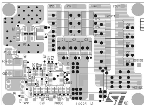
Figure 11. Power & signal plane
