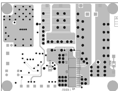
Figure 10. Internal ground plane
