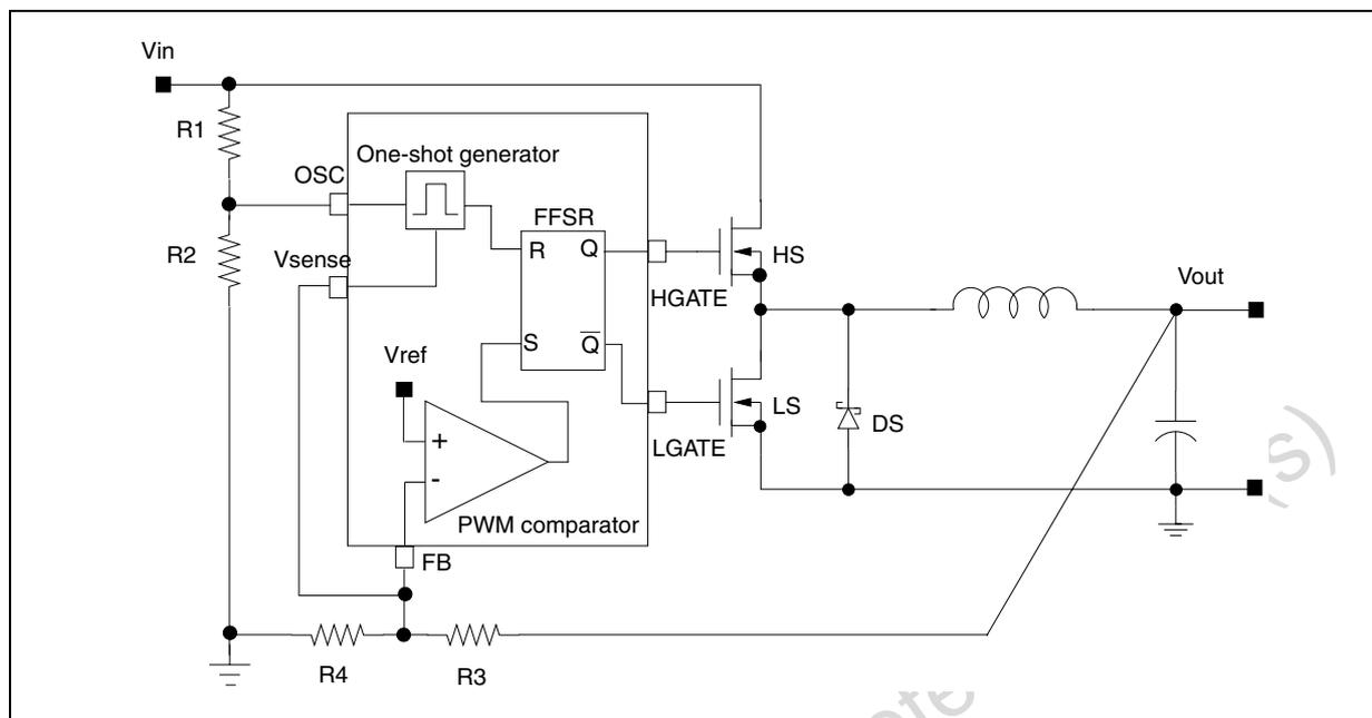
The device implements a Constant On Time control scheme, where the  $T_{ON}$  is the high side MOSFET on time duration forced by the one-shot generator. The on time is directly proportional to  $V_{SENSE}$  pin voltage and inverse to  $V_{OSC}$  pin voltage as in Eq1:
