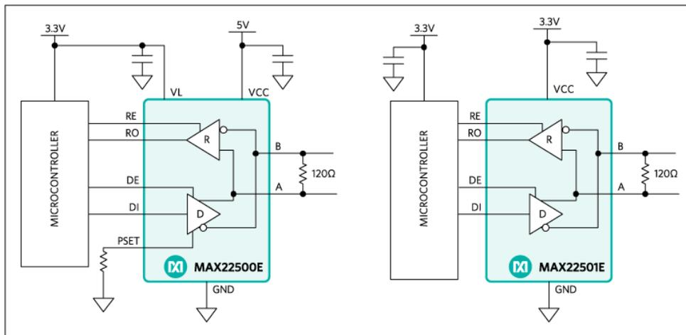
Figure C. MAX22500E and MAX22501E application circuits.
