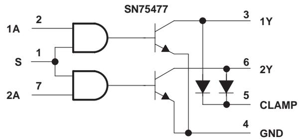
Positive Logic:  $Y = \overline{AS}$  or  $\overline{A+S}$
