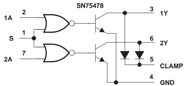
Positive Logic:  $Y = A+S$  or  $\overline{\overline{A} \overline{S}}$
