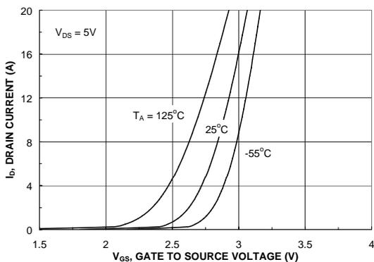
Figure 5. Transfer Characteristics.
