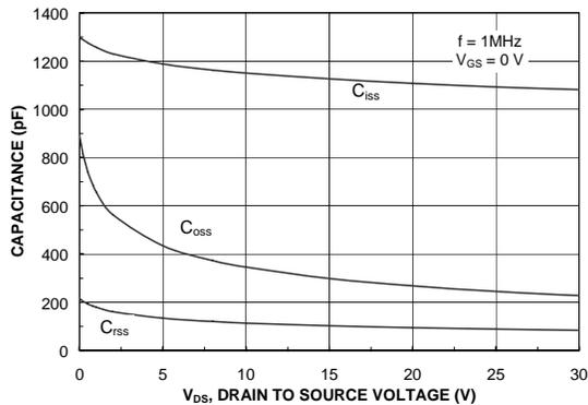
Figure 8. Capacitance Characteristics.
