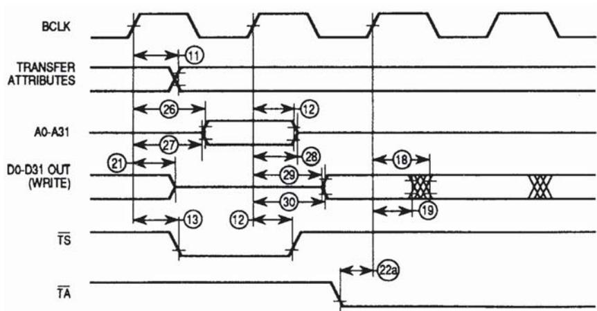
Figure 11. DLE Timing Burst Access
