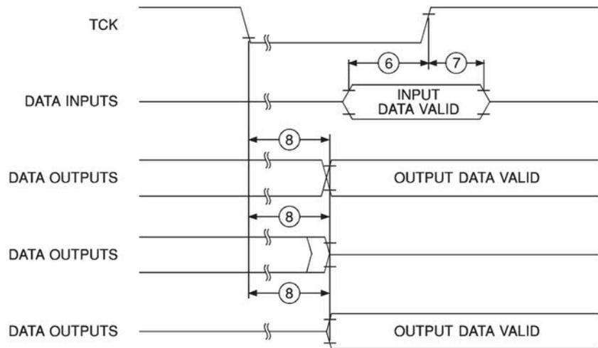
Figure 19. Test Access Port Timing Diagram
