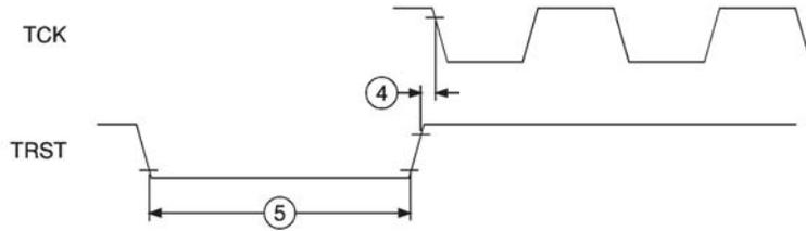
**Figure 18.** Boundary Scan Timing Diagram
