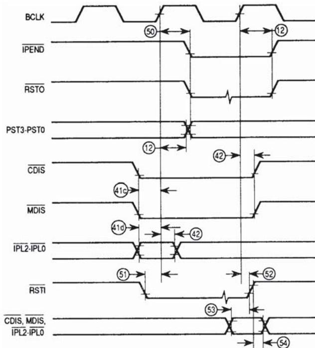
**Figure 16.** Clock Input Timing Diagram
