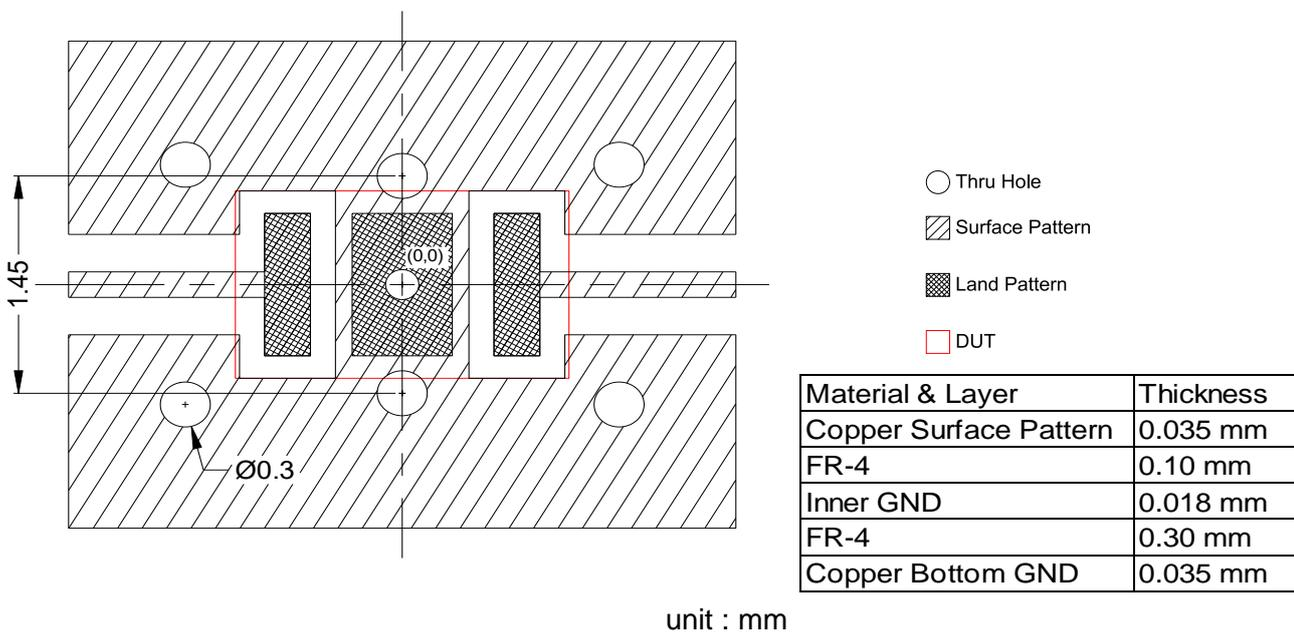
\* Line width should be designed to match 50 ohm characteristic impedance depending on PCB material and thickness.
