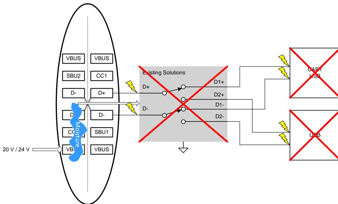
Figure 17. Existing Solution Being Damaged by a Short
