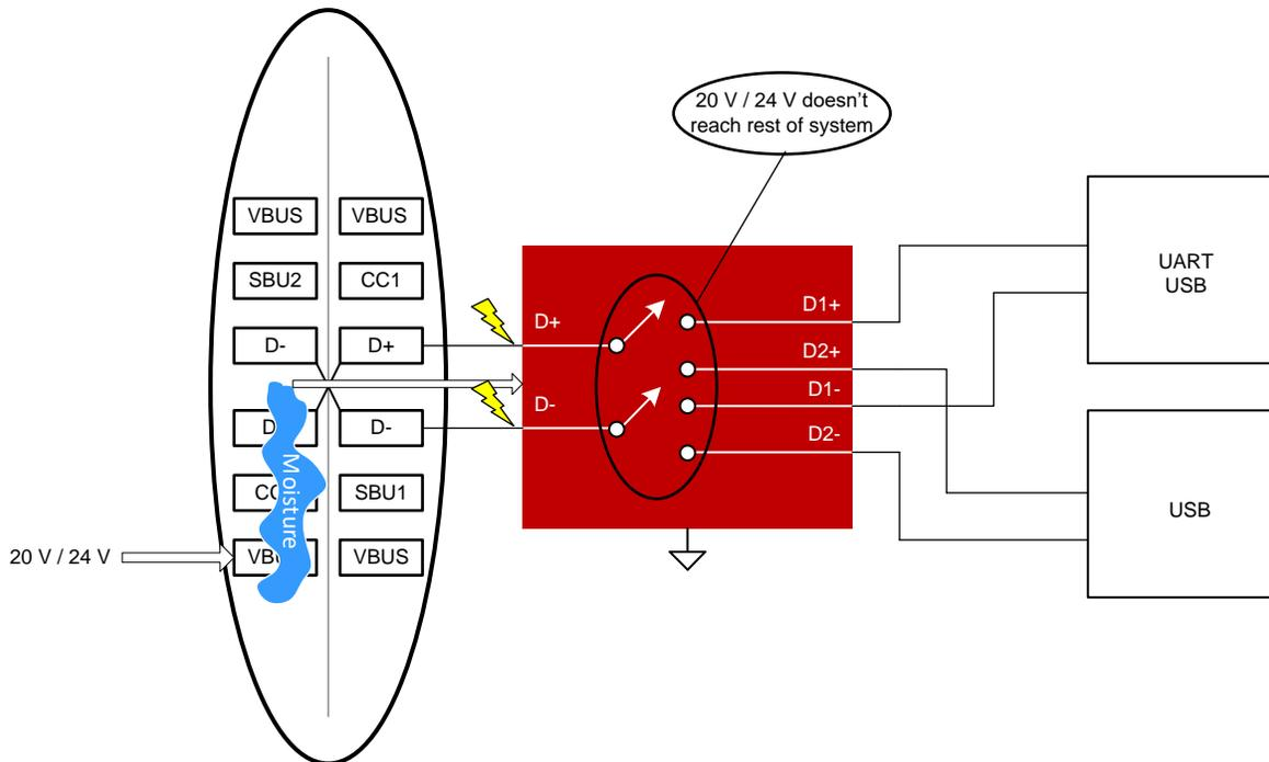
**Figure 18. Protecting During a 20-V / 24-V Short**
