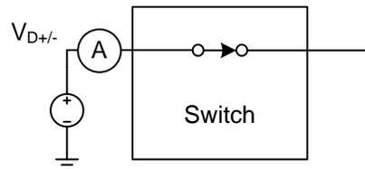
**Figure 7. On Leakage**
