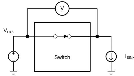
Channel ON,  $R_{ON} = V/I_{SINK}$
