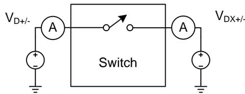
**Figure 6. Off Leakage**
