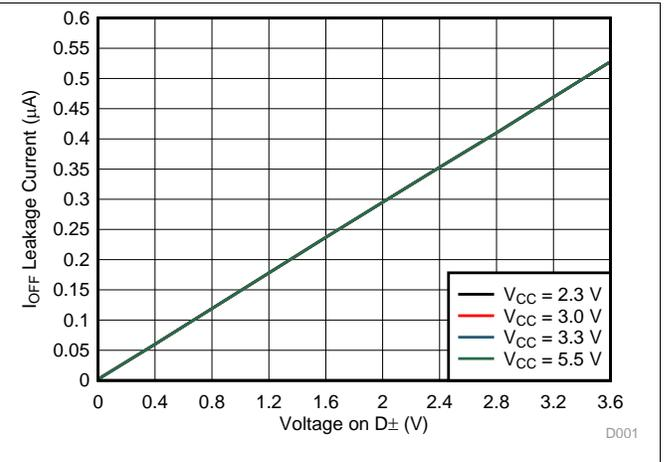
Figure 2.  $I_{OFF}$  Leakage Current vs Voltage on  $D_{\pm}$
